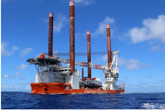
Figure 3.12: Jack-up crane vessel in transition. [18]
