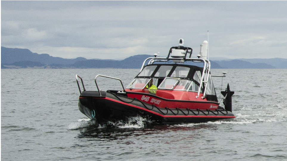
Figure 1.1: USV Telemetron autonomously driving during tests in the Trondheimfjord with a safety pilot (Courtesy of Maritime Robotics).
