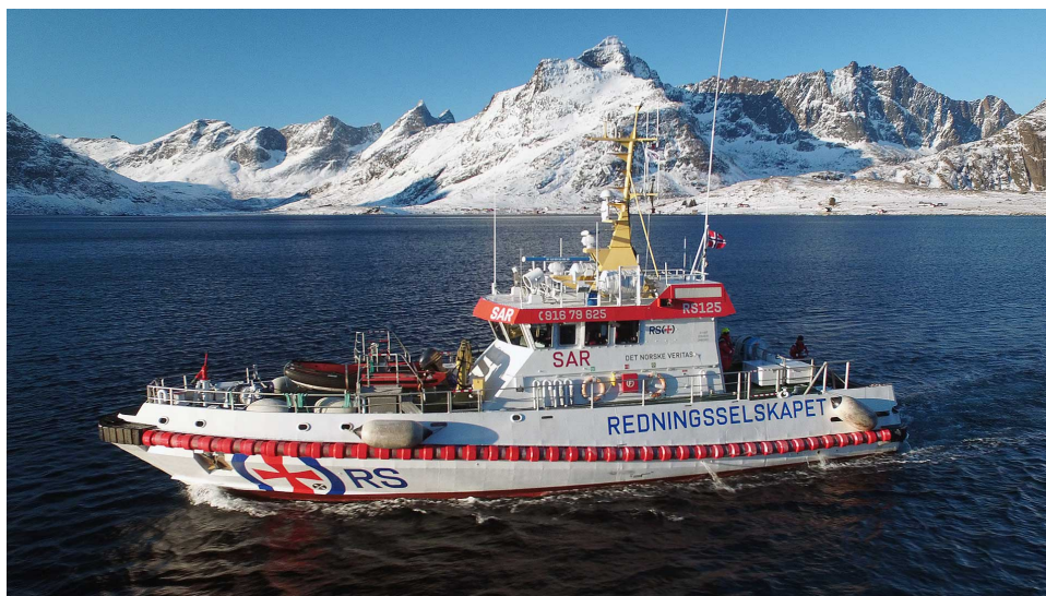
Figure 4.9: The rescue ship "RS 125 DNV" which is one out of six ships in the ship class "Fosen", providing the largest bollard pull power of 23 tonnes. Picture courtesy of https://www.redningsselskapet.no/ .
