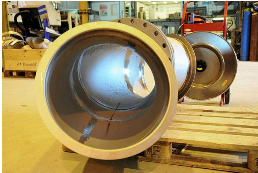
Figure 5.5: Bend inside a rigid part of a fish tube [159].
