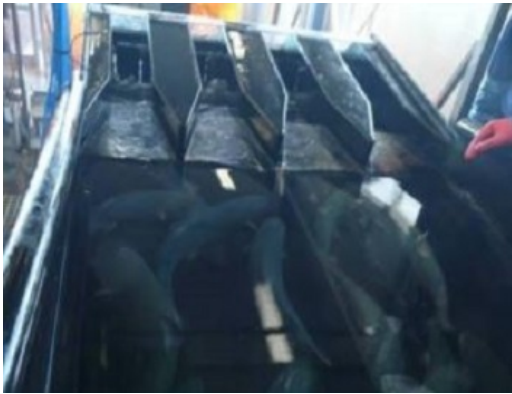
(a) The inlet side of a percussion machine.
