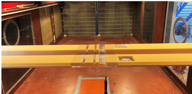
Figure 3.1: Complete wind tunnel model.
