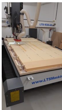
Figure 3.10: Milling of the inside geometry of the model.
