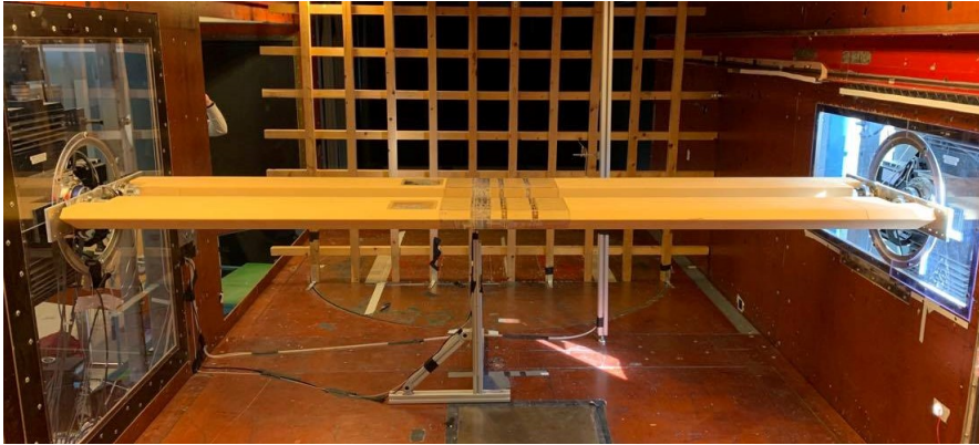
Figure 3.17: Model mounted in wind tunnel
