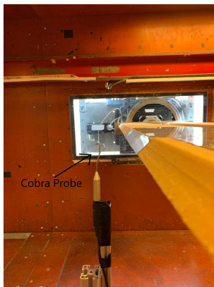
(a) Cobra Probe setup
