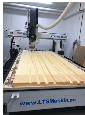
Figure 3.10: Milling of the inside geometry of the model.
