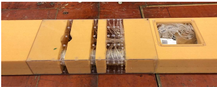
(c) Finished section model with tubes, Lexan plates and pressure scanners
