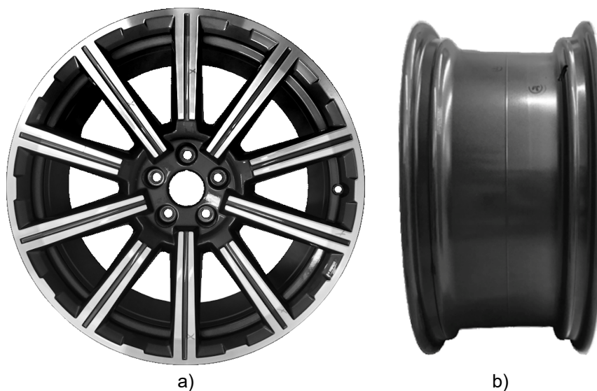
Figure 2.3: 2017 Audi Q7 ALY58988 rim, a) top view showing the short spoke configuration, b) side view. Modified version of image found in [4].
