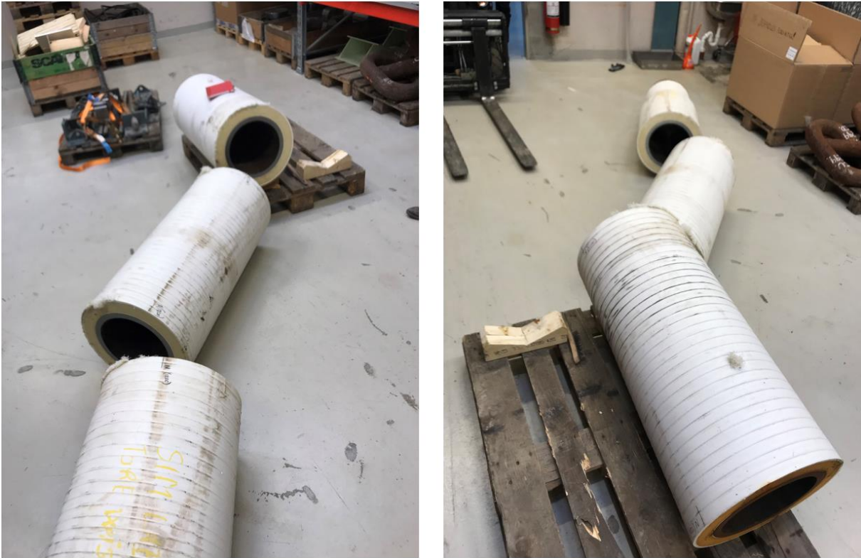
Figure A.3: Aligning the pipe-stubs to define cross-sectional orientation equal for all of them.
