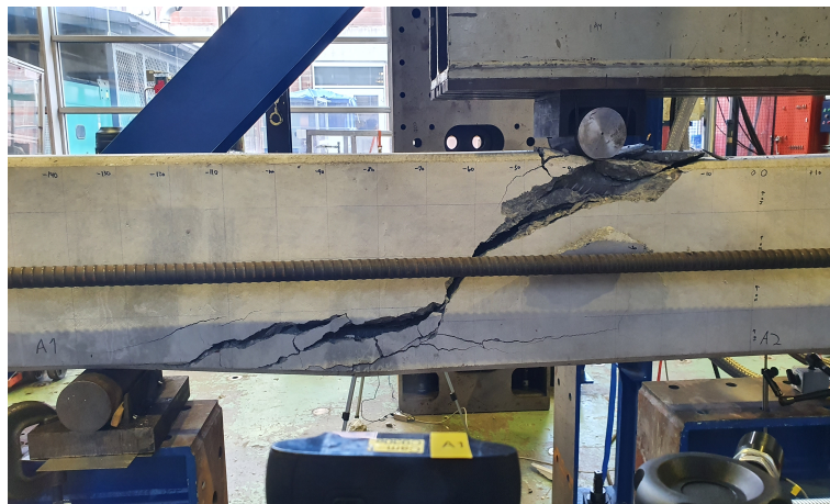
Figure D.9: Shear crack in B4 after the second peak in the load - displacement graph.
