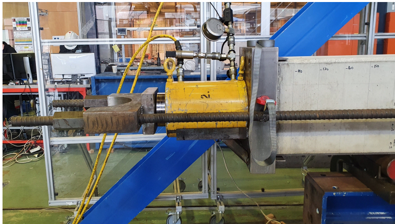
Figure 10: The axial load was applied using a jack and steel plates.
