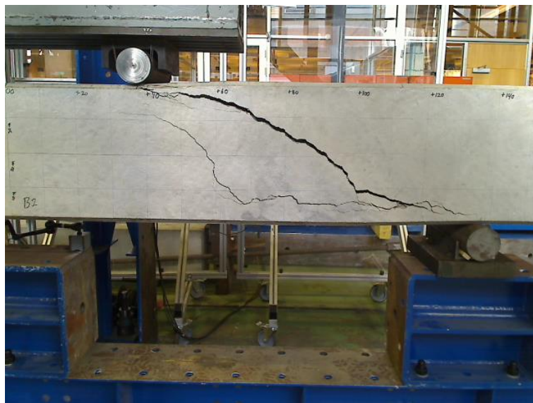
Figure D.2: Shear crack in B1 after the second peak in the load - displacement graph.
