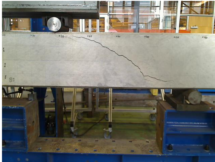
Figure D.1: Shear crack in B1 in connection with the first peak in the load - displacement graph.
