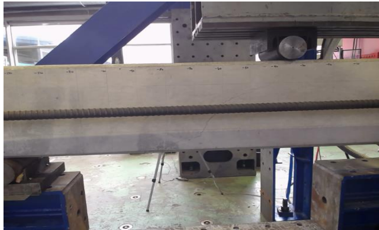
Figure D.7: Shear crack in B4 in connection with the first peak in the load - displacement graph.
