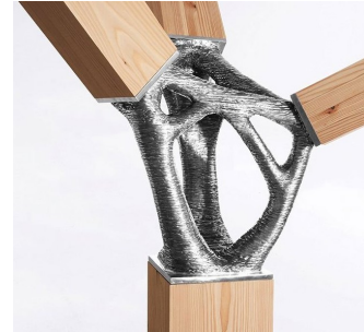
(c) A hollow steel joint in development by MX3D and Takenaka. The shape is created using topology optimisation and thereafter 3D printed before filling the core with mortar. Photo: ©Leonard Fäustle (MX3D, 2020)
