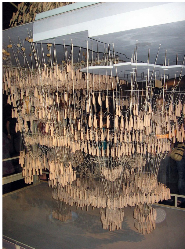
Figure 2.3: Hanging chain model of Colònia Güell [3].
