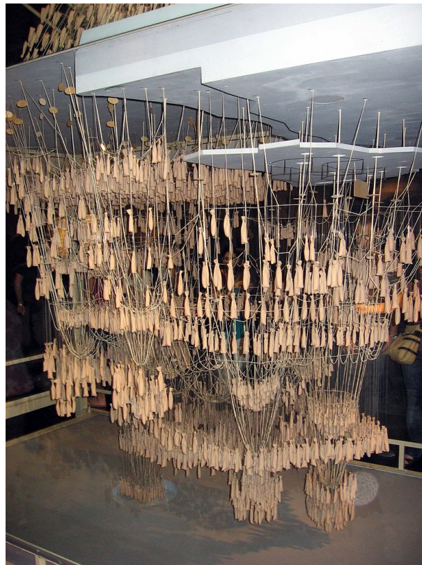
Figure 2.3: Hanging chain model of Colònia Güell [3].
