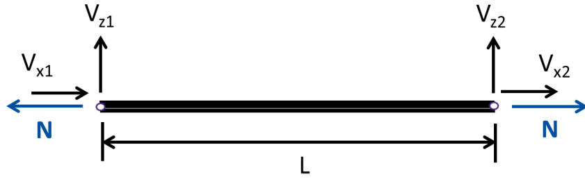
Figure 2.15: A two-noded bar element with 4 DOFs.
