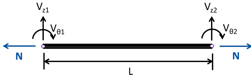
Figure 2.14: A two-noded beam element with 4 DOFs.
