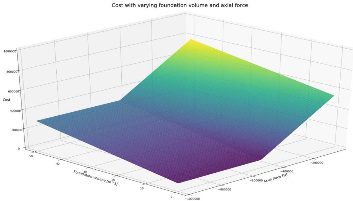
**Figure 4-5: Closeup on how cost varies dependent on foundation volume and axial force.**
