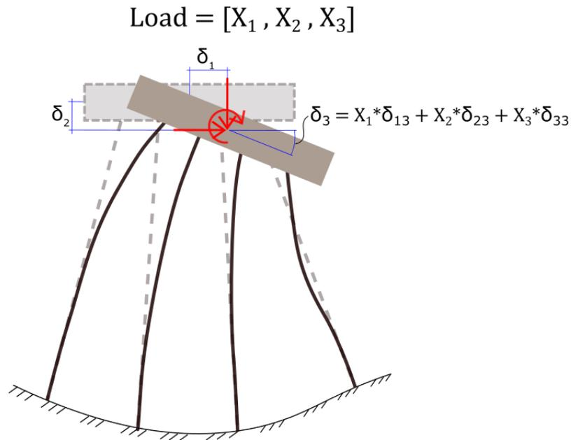
**Figure 6-2: Combined action from an arbitrary load.**
