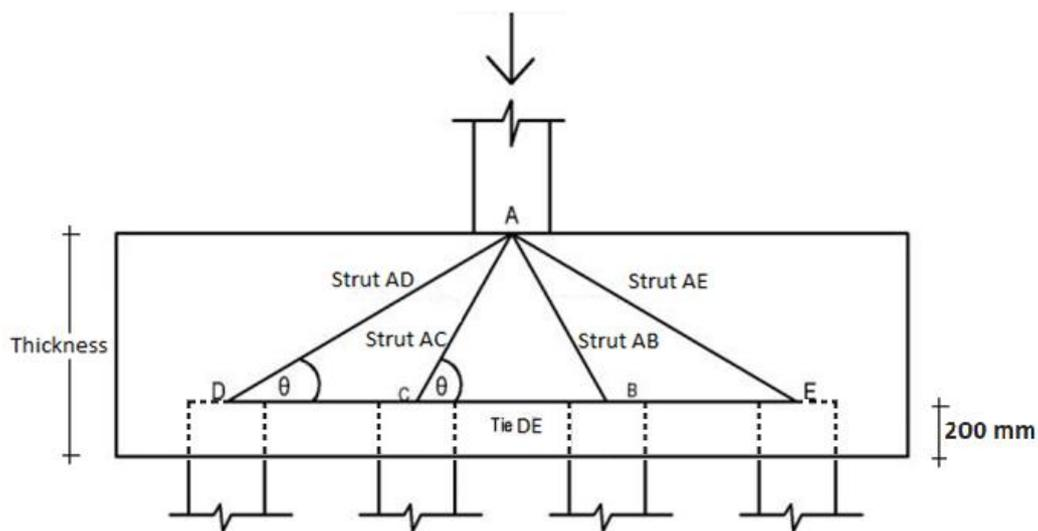
Figure 4-2: Strut and tie model of pile foundation.
