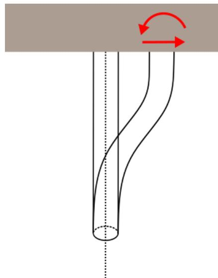
Figure 3-9: Illustration on the lateral carrying capacity of a pile.
