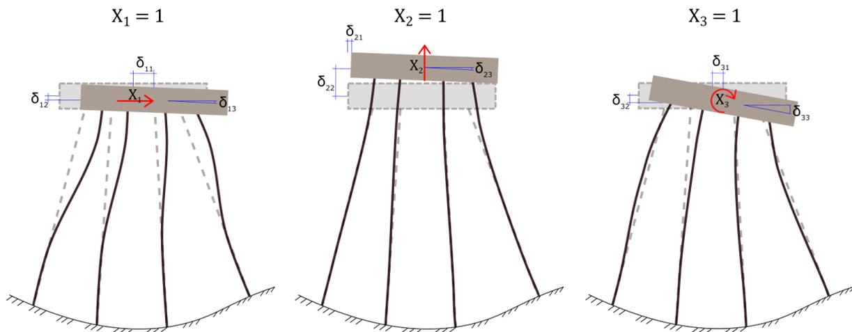
Figure 6-1: Explanation of the unit load method.
