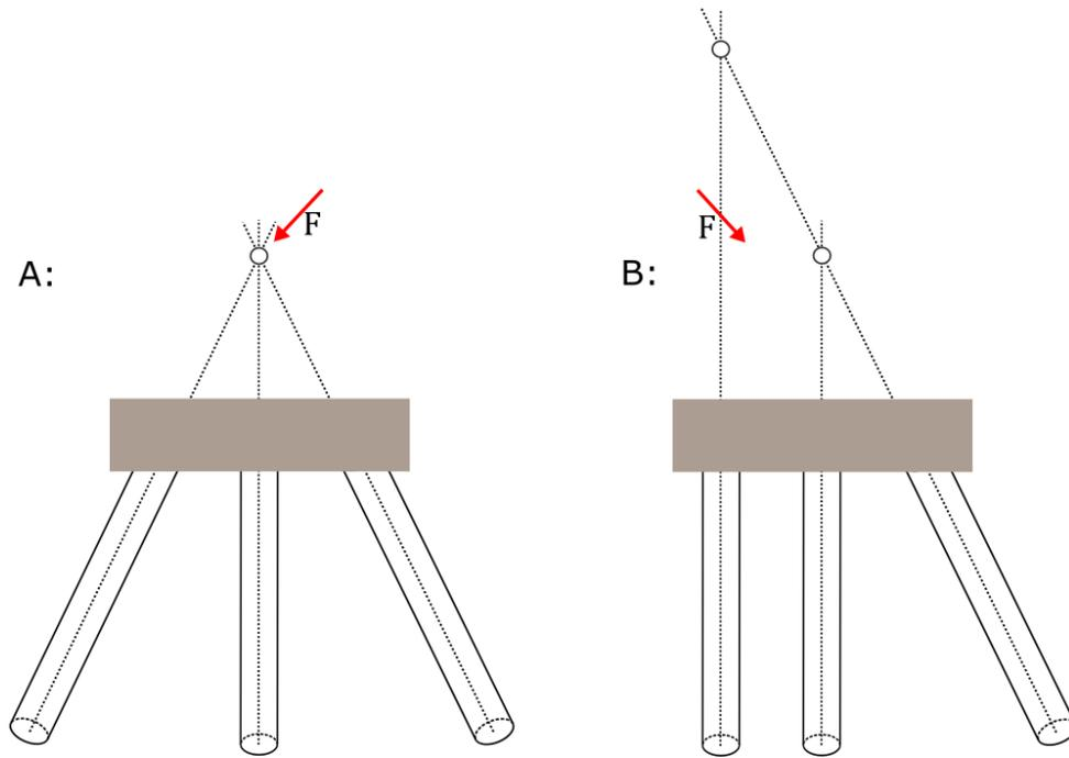
Figure 3-11: Example of an unstable (A) and stable (B) configuration.
