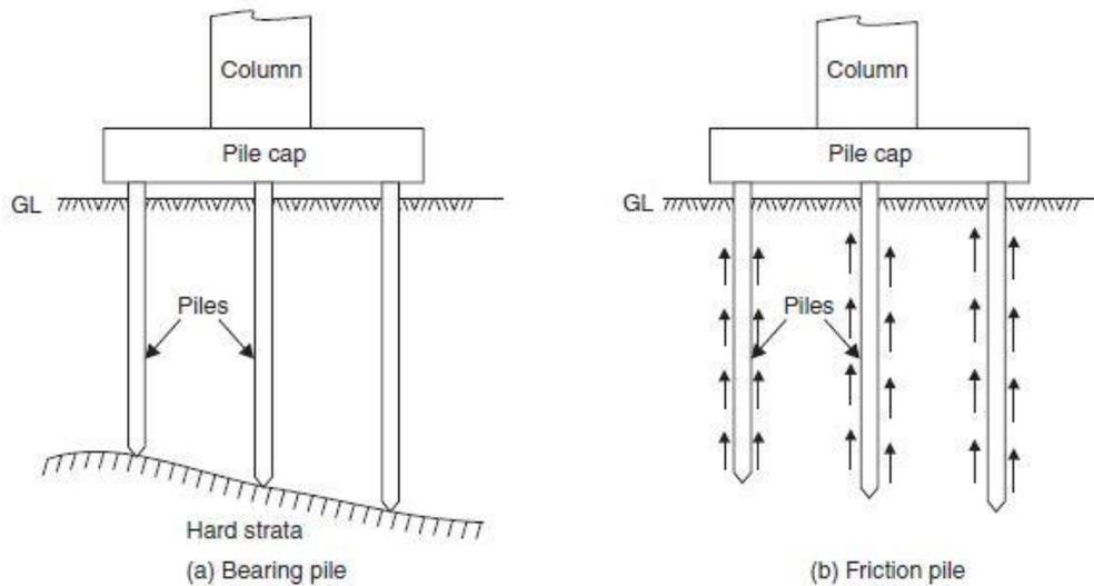
**Figure 3-7: Pile foundation with the two different carrying methods.**
