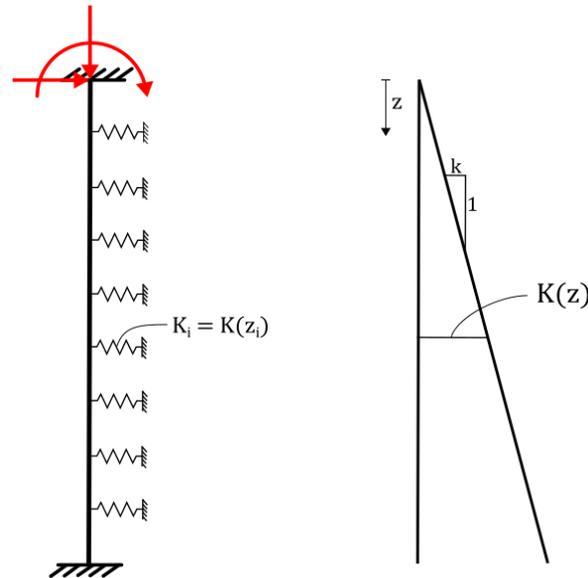
Figure 3-5: Calculation model of a pile, with lateral springs.
