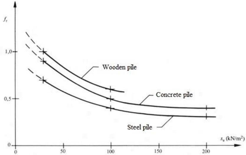
Figure 3-2: Reconsolidation factor as a function of shear resistance and pile type [17].
