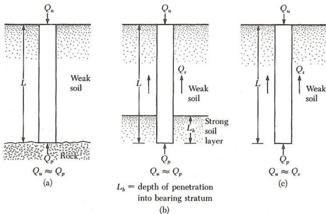
Figure 3-1: Different load carrying categories; point bearing pile (a), combination of point bearing and friction pile (b) and friction pile (c) [19].
