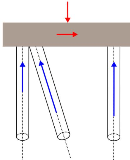
Figure 3-8: Illustration on how loads are carried as axial loads in piles.
