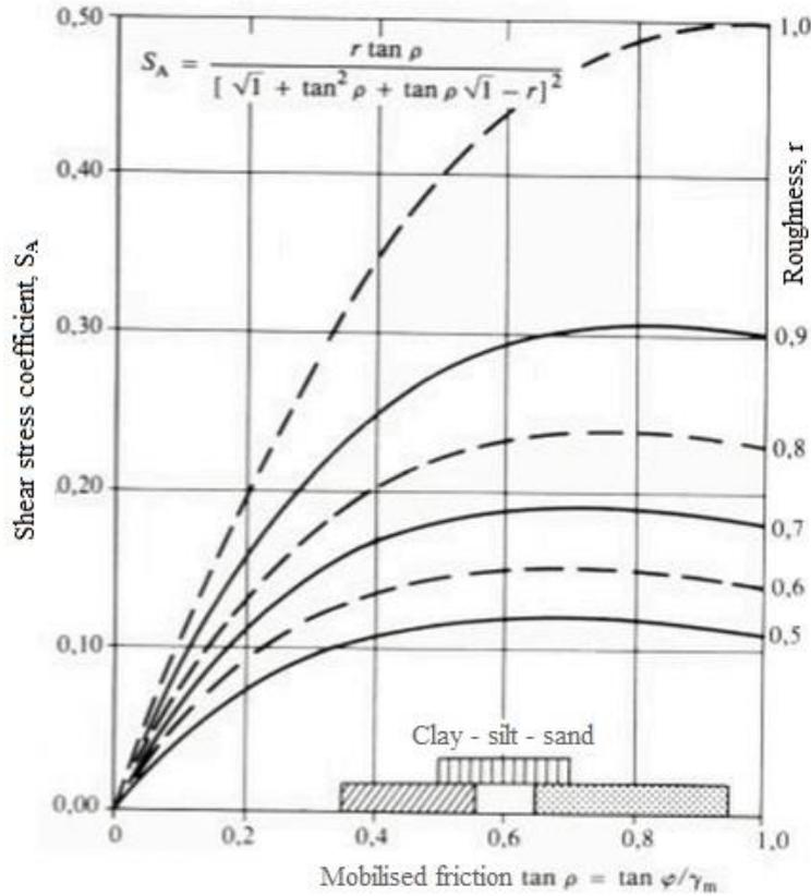
Figure 3-3: Shear stress coefficient as a function of roughness and mobilised friction [17].
