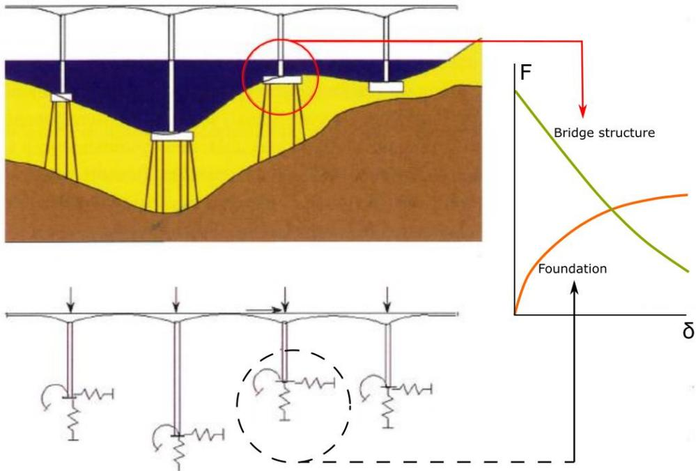
Figure 3-12: Illustration of the system model for piled bridges subjected to static forces [11].
