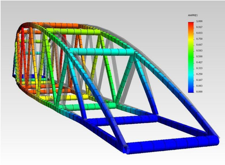
Figure 1-3: FEA result of a bridge [4].
