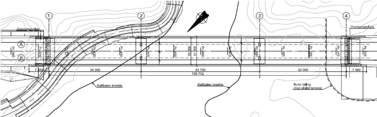
Figure 1-7: Plan view of Råna bridge.
