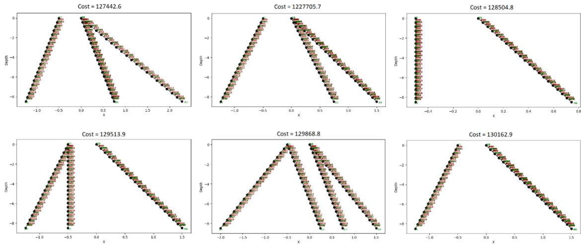
Figure 5-4: low cost solutions from second analysis (with constrains).
