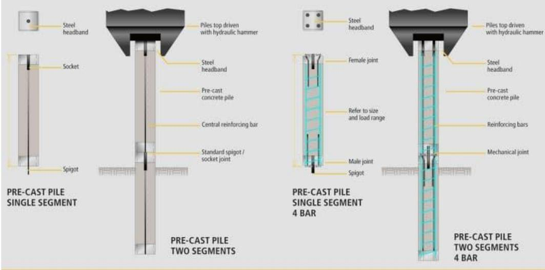
Figure 3-6: Precast concrete pile with detailing [21].
