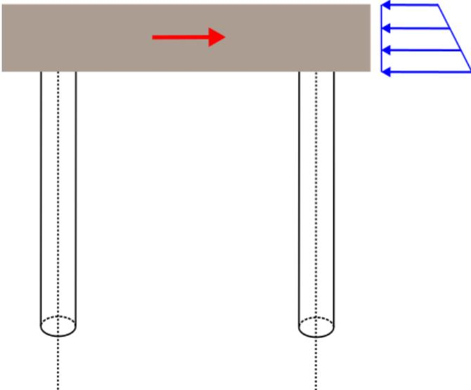
Figure 3-10: Illustration on the lateral carrying capacity from the slab.
