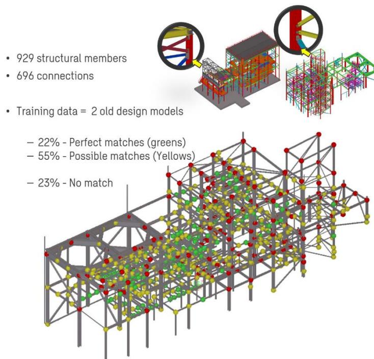
Figure 1-5: Structure where ML was used for steel connection design [8].
