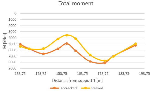
Figure 8.9: Total moment in outer beam Solid model
