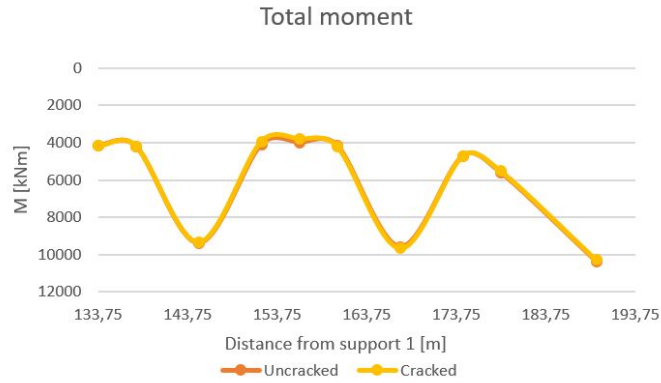
Figure 8.5: Moment distribution between the beams Frame model
