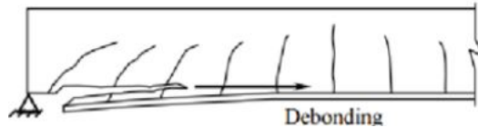
Figure 3.12: Debonding due to concrete cover separation [26]
