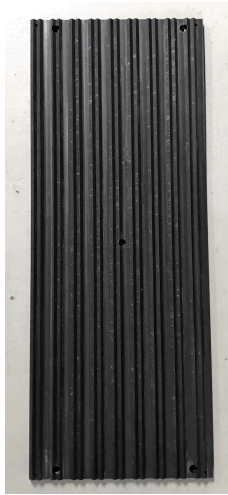
Figure 4.8: The corrugated mould used to shape the aluminium mesh spacers.
