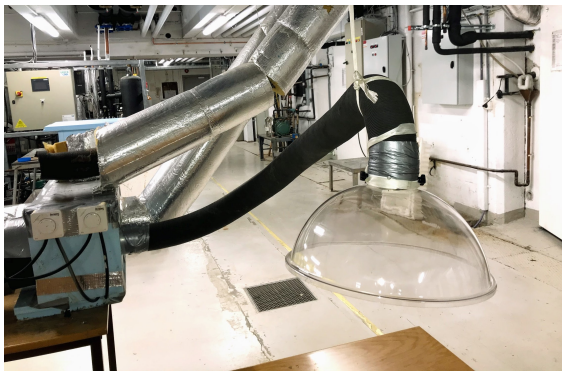
Figure 5.1: Ventilation hood connected to the exhaust air inlet.
