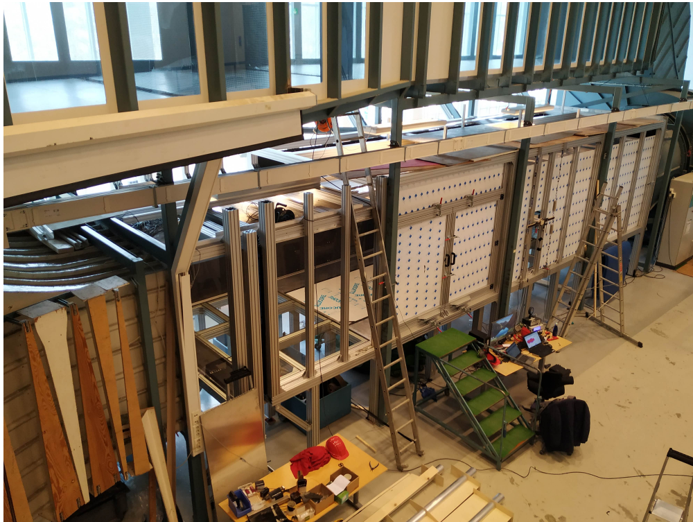
Fig. B.5 The newly refurbished wind tunnel test-section. Image courtesy of Magnus Kyrkjebø Vinnes.
