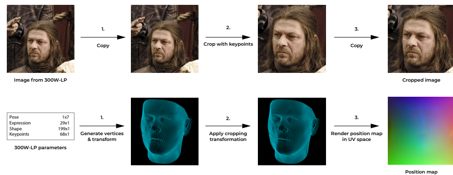
Figure 4. The 300W-LP training data generation pipeline. The pipeline in the top row corresponds to a pre-processing procedure and is related to the 2D data. In the pre-processing, the image is cropped based on the provided key-points and the crop parameters were kept. The pipeline in the second row represents the actual generation of the 3D training data. First, the vertices are generated and transformed to the correct pose using the face3d library. Then, the vertices are cropped according to the crop parameters that were previously extracted. Finally, the position is rendered map in UV space.
