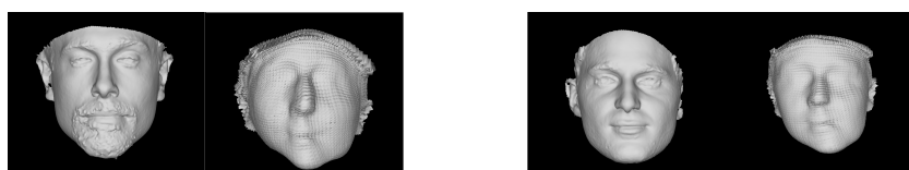
Figure 19. Two 3D facial meshes from the MICC Florence dataset (left part of each pair) compared to the reconstructed 3D facial meshes made by the synthetically trained 2-input network (right part of each pair).
