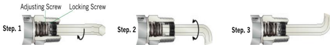
Figure 4.5: Cracking pressure adjustment.
