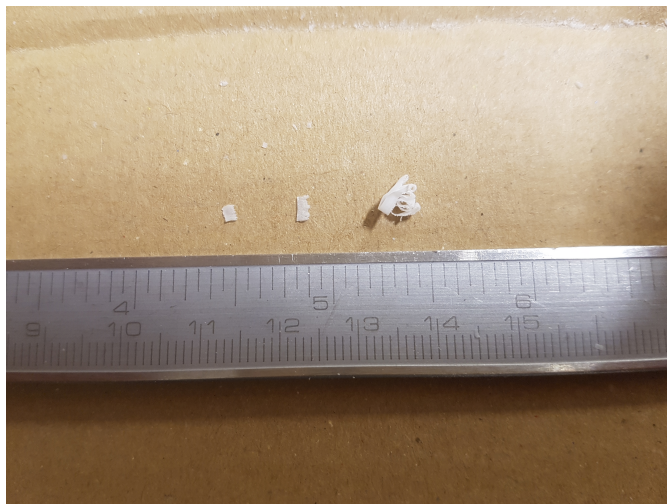
Figure 4.5: Sizes of the Plexiglas particles with with a caliper as reference. The unprocessed shavings is seen to the right, the first size reduction in the middle and the final reduction step to the left.
