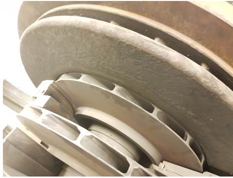
Figure 3.2: Close up of impeller and diffuser hub side of a multistage hydrocarbon compressor previously operating at Åsgård.
