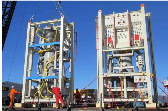
Figure 1.1: Gullfaks C wet gas compressor [2].
