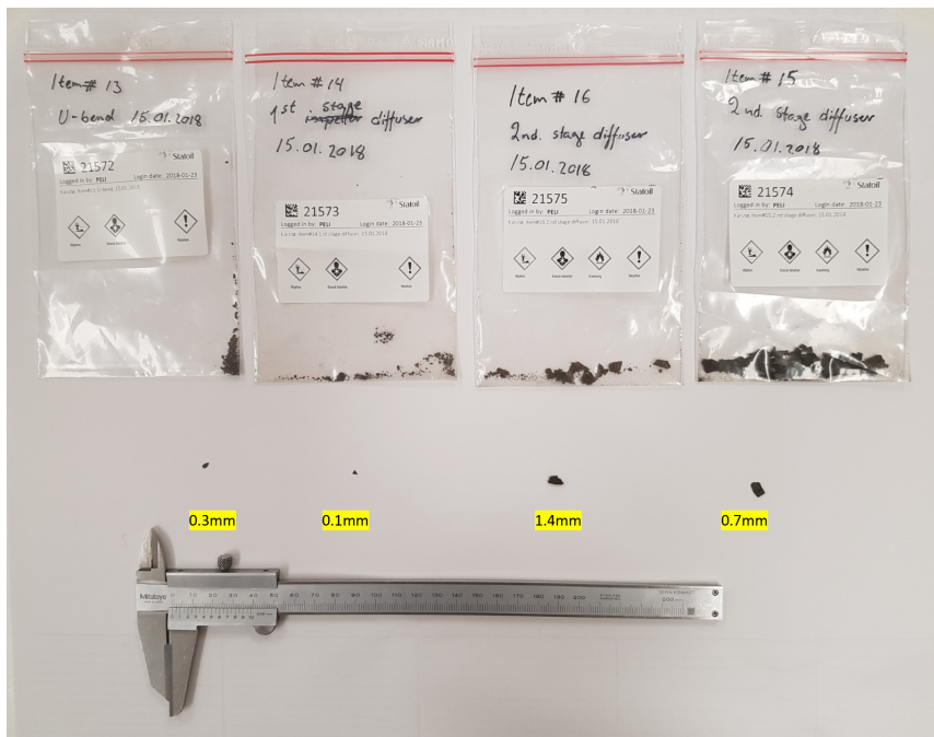
Figure 4.2: Deposits collected from different components of a hydrocarbon compressor at K-lab. The different samples, from left to right, were obtained from respectively: the U-bend, 1 st stage diffuser, and two locations of the 2 nd stage diffuser. The thickness of the deposits from the different compressor parts are highlighted in yellow.
