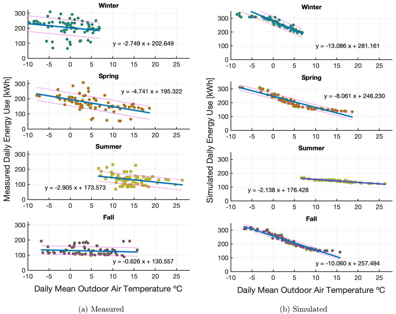
Figure 7.12: Arne Rønning Seasonal Analysis of Measured and Simulated Energy Use
