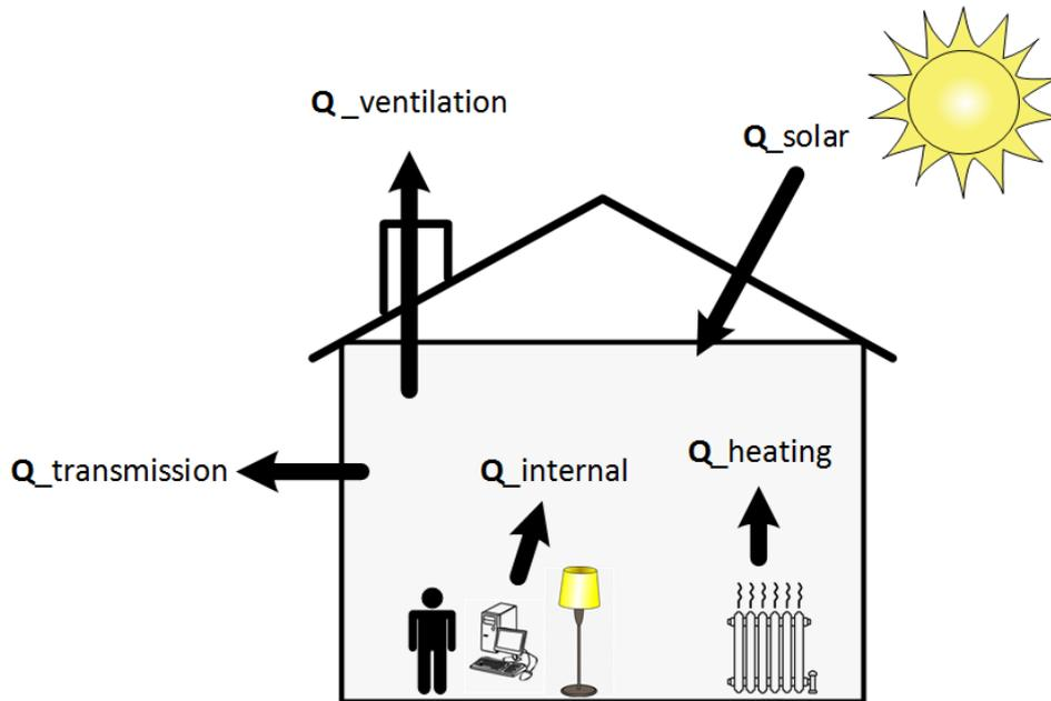
Figure 2.3: Principle Sketch of Heat Balance
