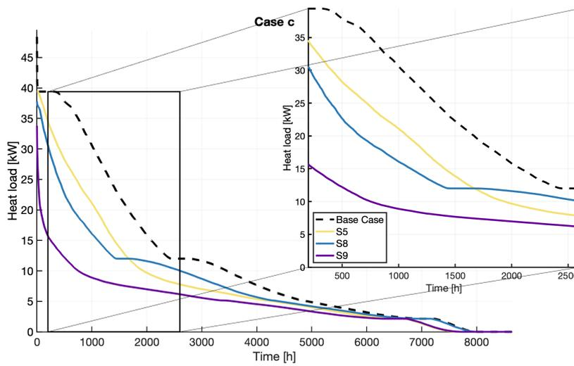
Figure 7.19: Rehabilitation Heat Duration Curve: Case c
