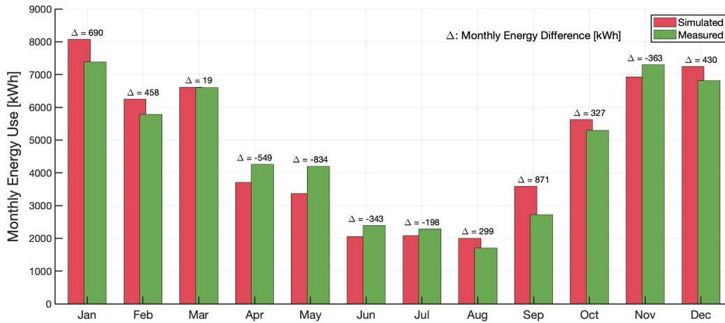
Figure 7.9: HUS Ark L4 Measured vs Simulated: Monthly Energy Use
