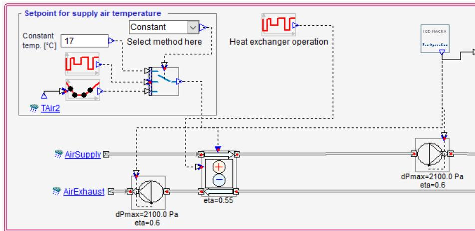
Figure 5.5: AHU Schematics in IDA ICE
