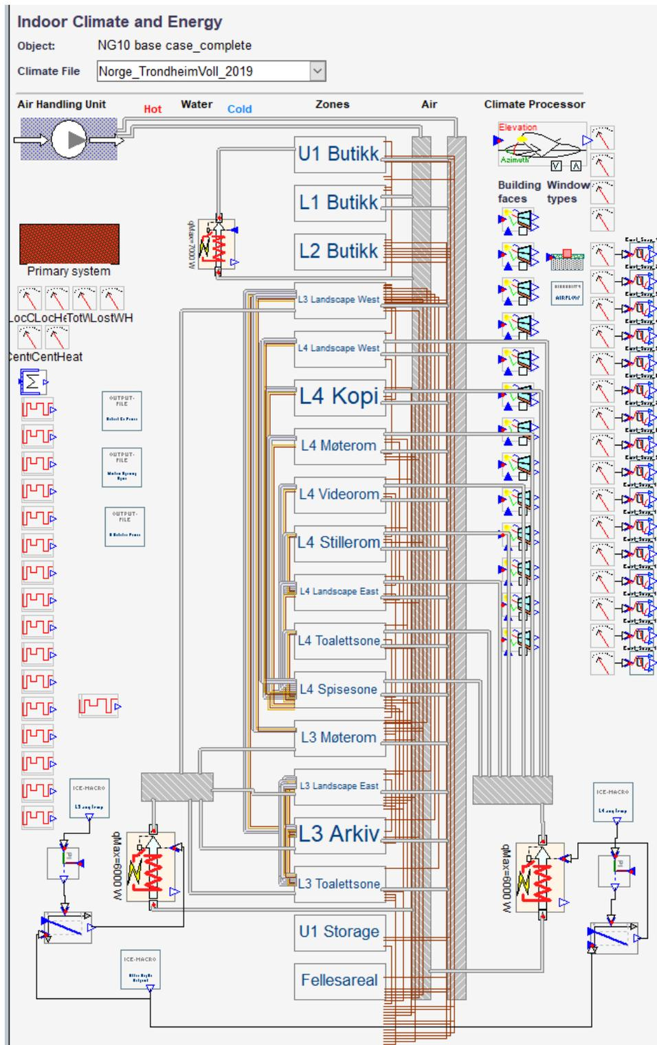
Figure C.1: Base Case Schematics Mode Interface
