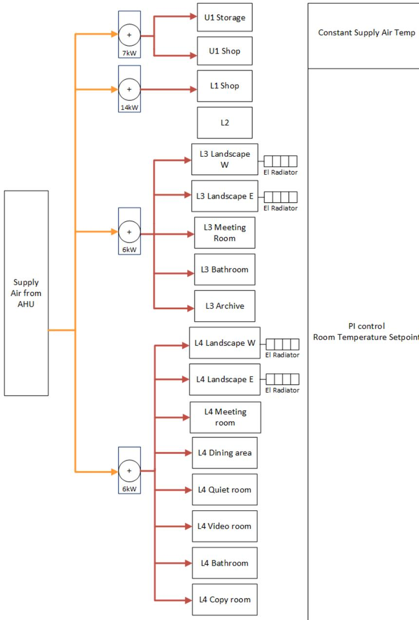
Figure 5.6: Principle Sketch of Modelled Heating System in Base Case
