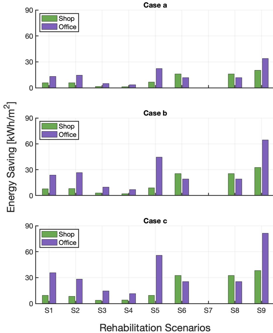
Figure 7.15: Heat Energy Saving for Rehab Scenarios
