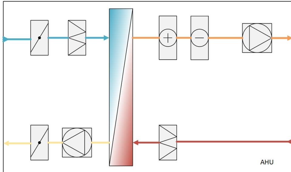
Figure 2.6: Principle Sketch of AHU
