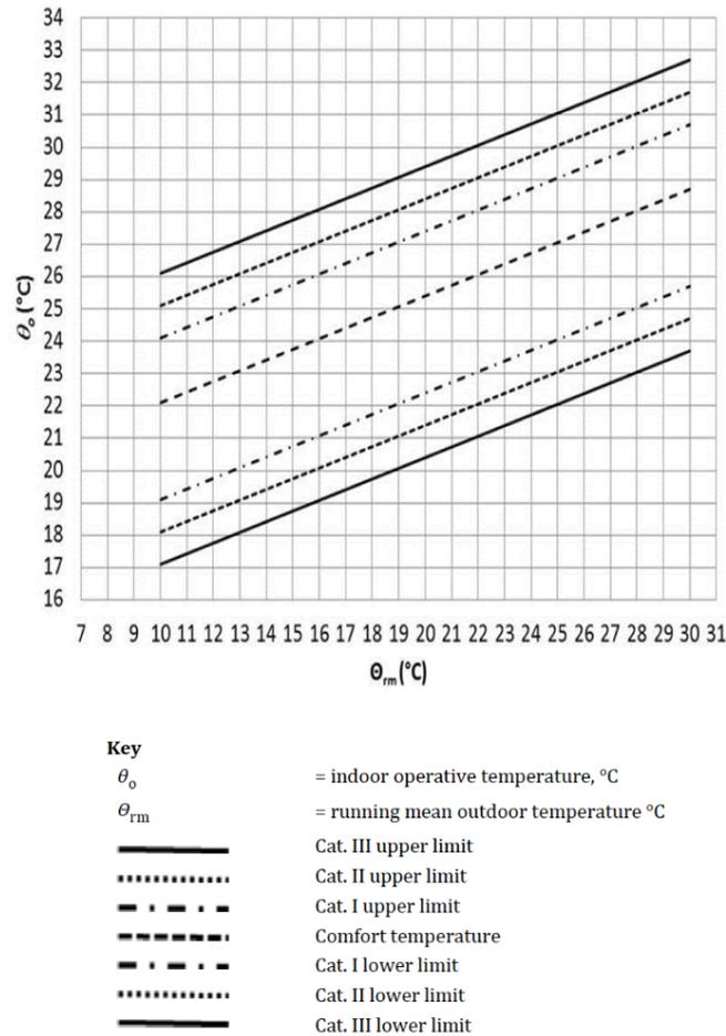
Figure 2.5: Acceptable Temperature Ranges for Thermal Comfort [2]
