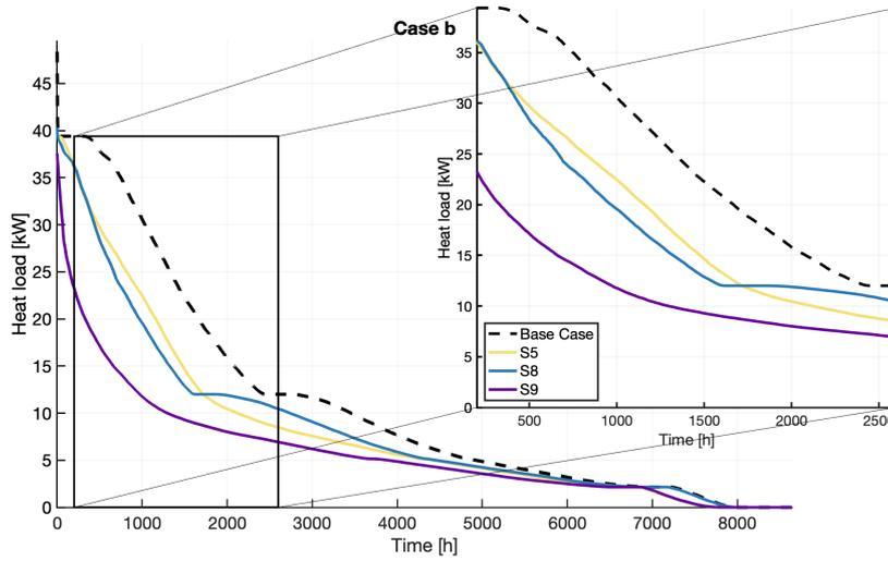
Figure 7.18: Rehabilitation Heat Duration Curve: Case b
