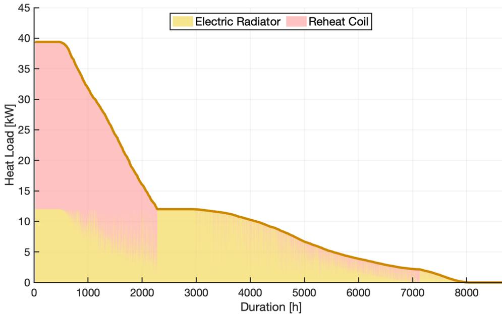
Figure 7.6: Base Case Heating Duration Curve
