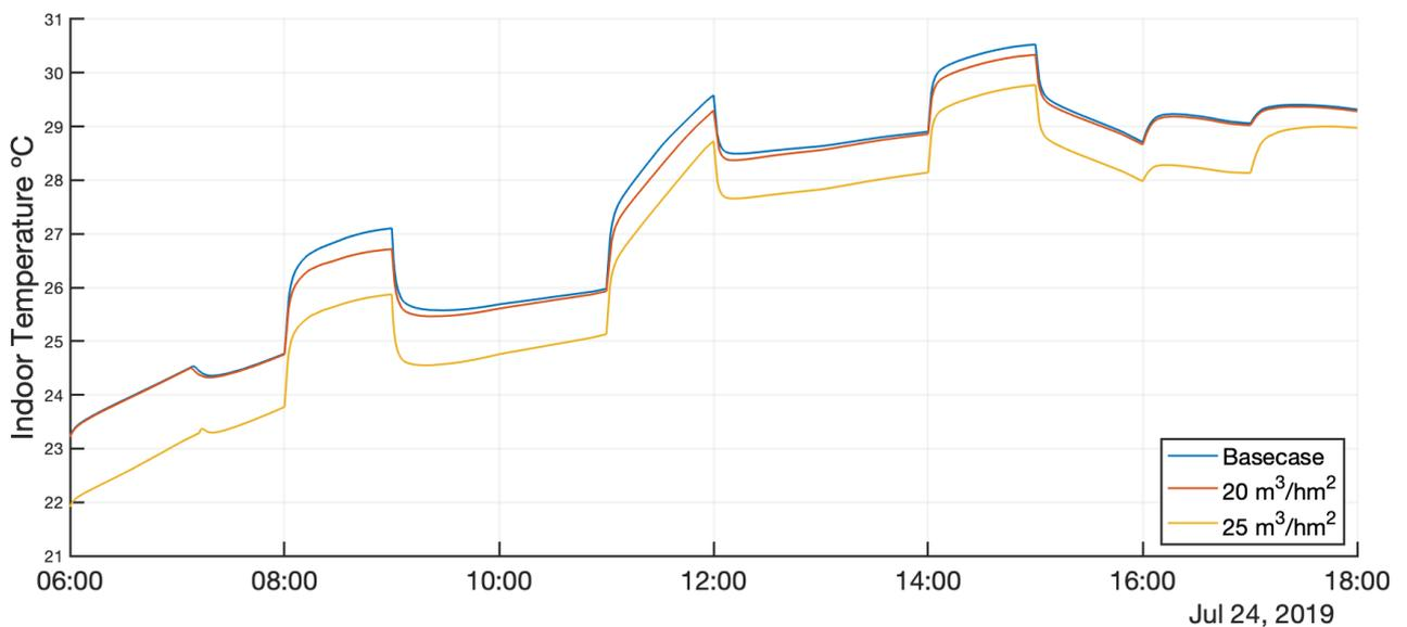
Figure 7.23: L4 Meeting Room Indoor Temperature With Improved Air Flow Rates
