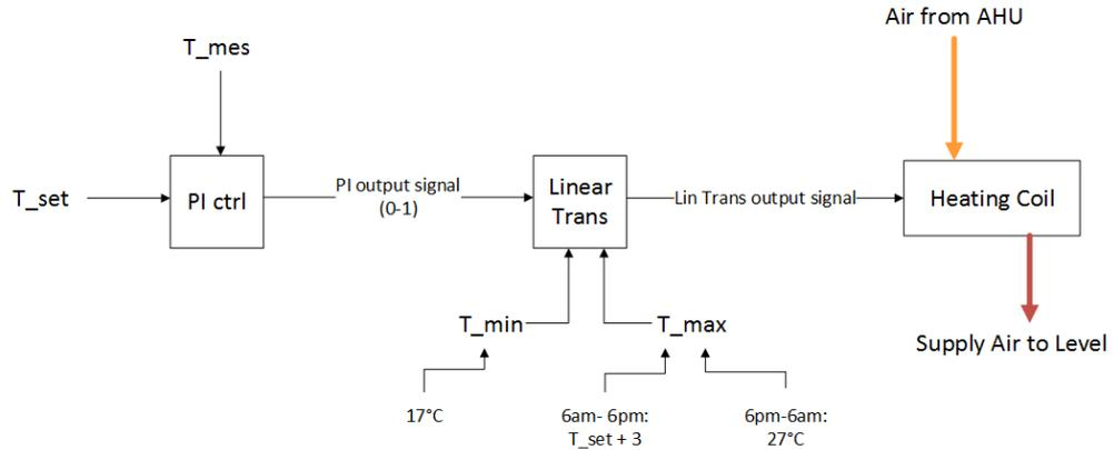
Figure 5.7: Reheat Coil Connection Diagram
