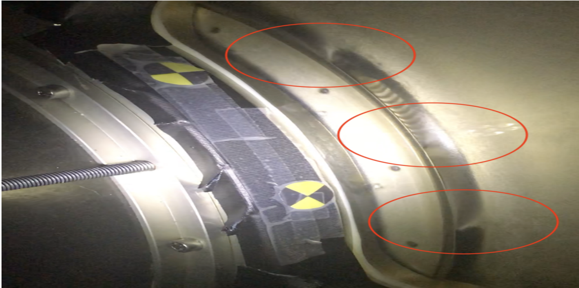
Figure 14: Impeller outlet water jet, NTNU Test Facility.
