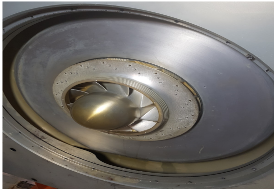
Figure 38: NTNU Test Facility diffuser.
