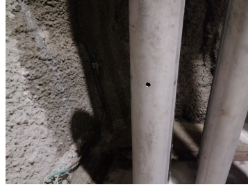
Figure 3.6: Hole drilled for measuring air velocity
