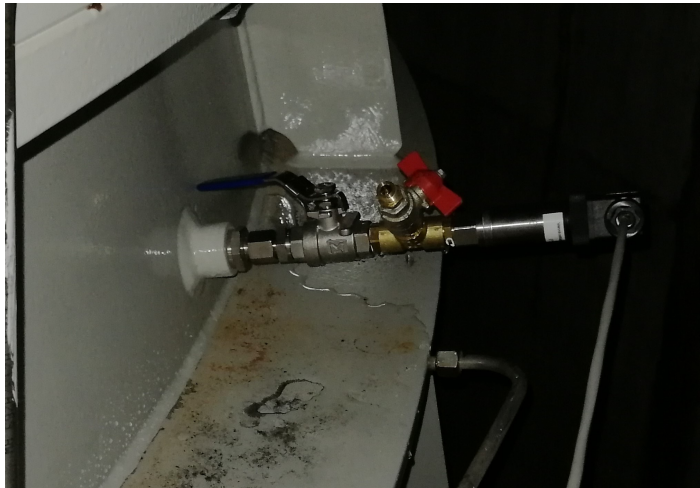
Figure 3.2: Draft tube pressure sensor 2, with the transition piece
