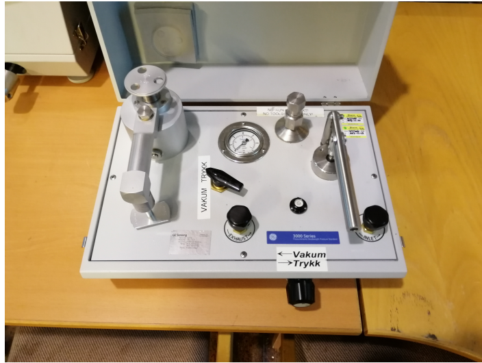
Figure 3.7: Low range dead weight tester
