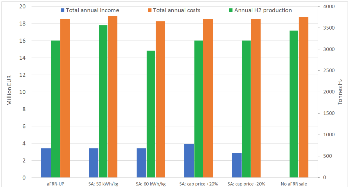
Figure 5.21: Sensitivity analysis results for a 45 MW electrolyser delivering up-regulating aFRR capacity in the German grid.
