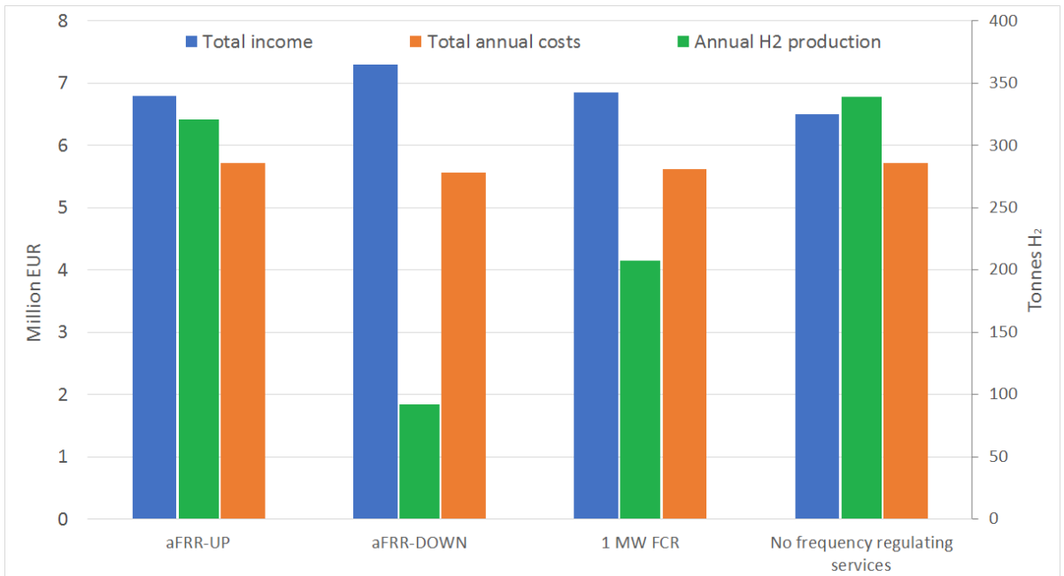
Figure 5.15: Analysis results for a 2.5 MW electrolyser operating in the German grid.
