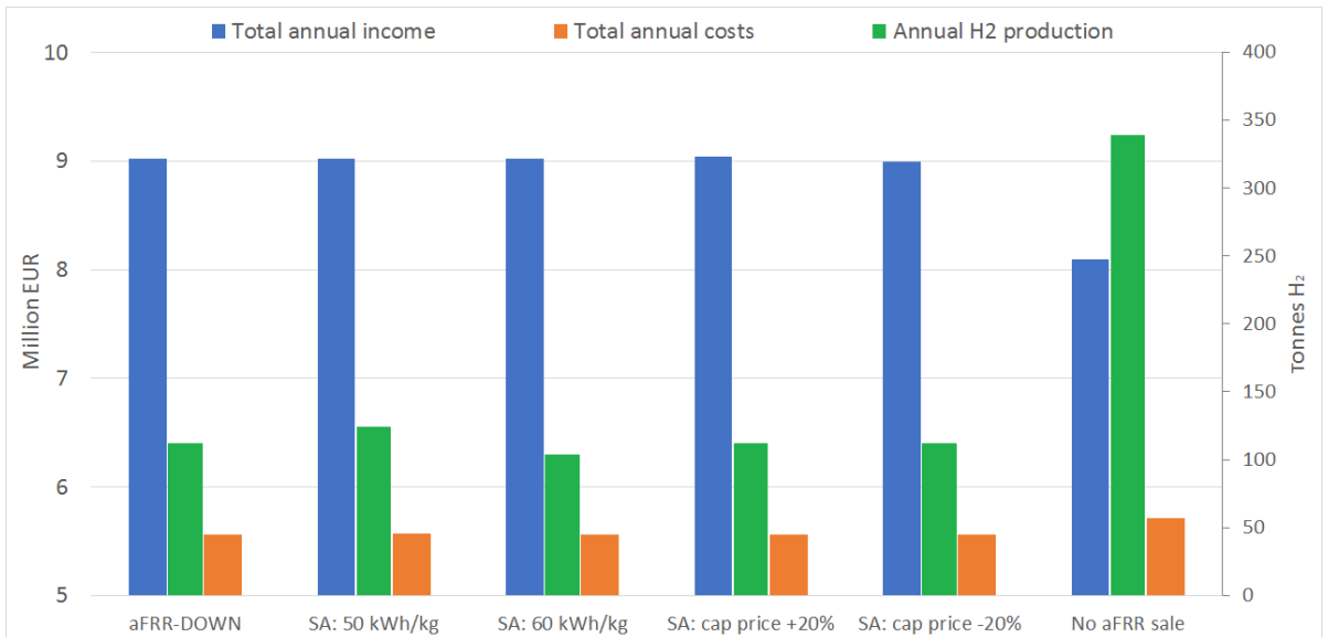
Figure 5.10: Sensitivity analysis results for a 2.5 MW electrolyser delivering down-regulating frequency restoration reserve capacity in the Spanish grid.
