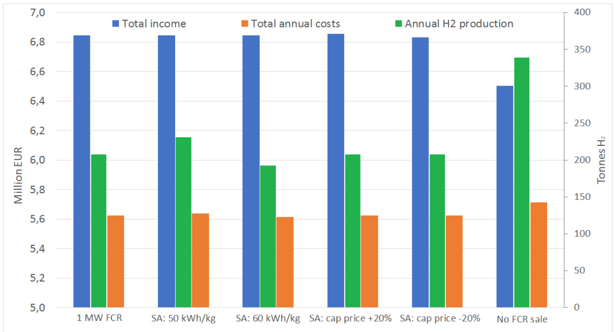
Figure 5.18: Sensitivity analysis results for a 2.5 MW electrolyser delivering FCR capacity in the German grid.
