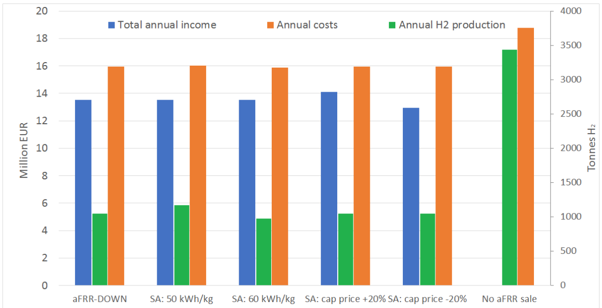
Figure 5.14: Sensitivity analysis results for a 45 MW electrolyser delivering down-regulating frequency restoration reserve capacity in the Spanish grid.
