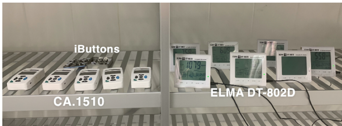
Figure 3.1: Instruments used in the field measurements. CA.1510 (in front, left), iButtons (back, left), and ELMA DT-802D (right)
