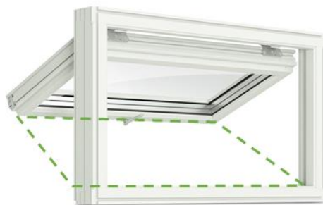
Figure 32: Illustration of window opening area of a rectangular top-hinged window.
