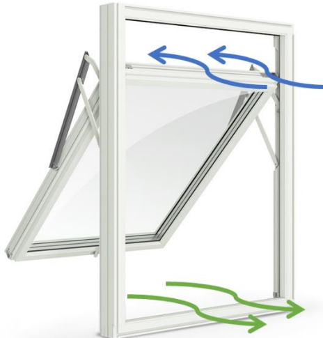
Figure 20: Illustration of how window opening can affect the effectivity of natural ventilation. The green arrows illustrate the fresh air that enters the room from outdoors, the blue arrows illustrate the mixed air which exits the room.
