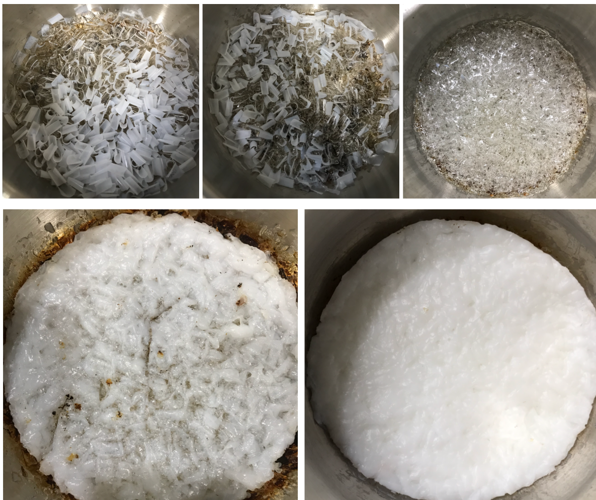
Figure 4.6: Top row: High-density polyethylene at different stages during melting. Bottom row: Solid high-density polyethylene after being melted at 140°C (left) and 220°C (right).
