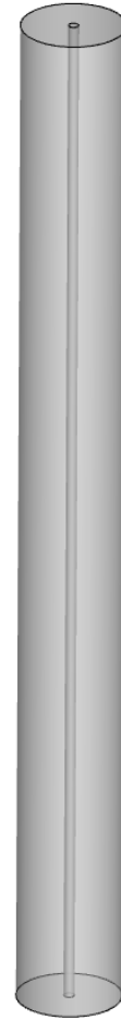
Figure 3.2: Geometry used for CFD simulations of a PCM cylinder with a wire along the center line.
