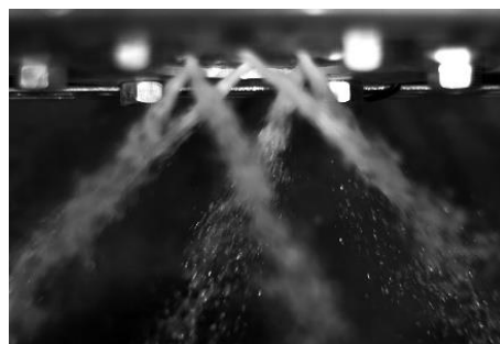
(b) Vortex injector exit using Water with a pressure drop of 30 bar
