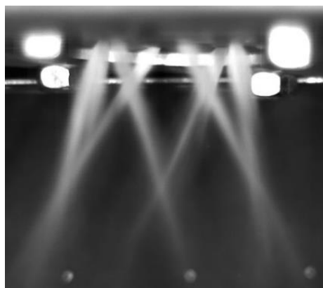
(a) Vortex injector exit using N_2O
