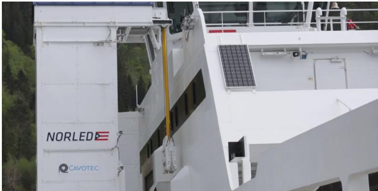
Figure 34 Charging solution on MF Ampere. Screenshot (Cavotec, 2016)
