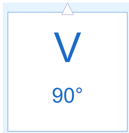
Figure 5-3: Volume function icon. The angle indicates that this function belongs to a control volume starting at a rotational angle of 90^\circ .
