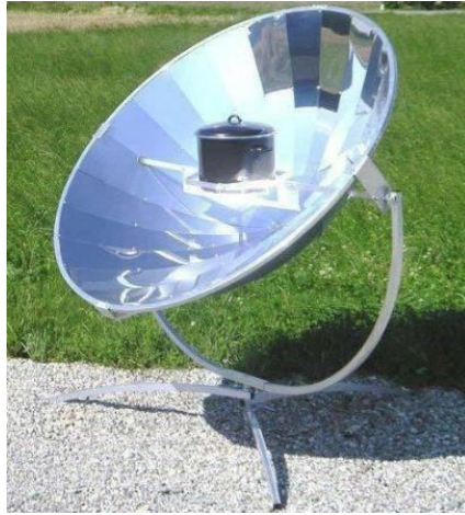
Figure 3.3 Concentrating type cooker (concentration from below) [34]
