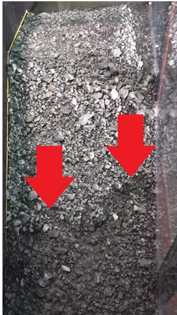
Figure 27 Internal erosion down stream test 1
