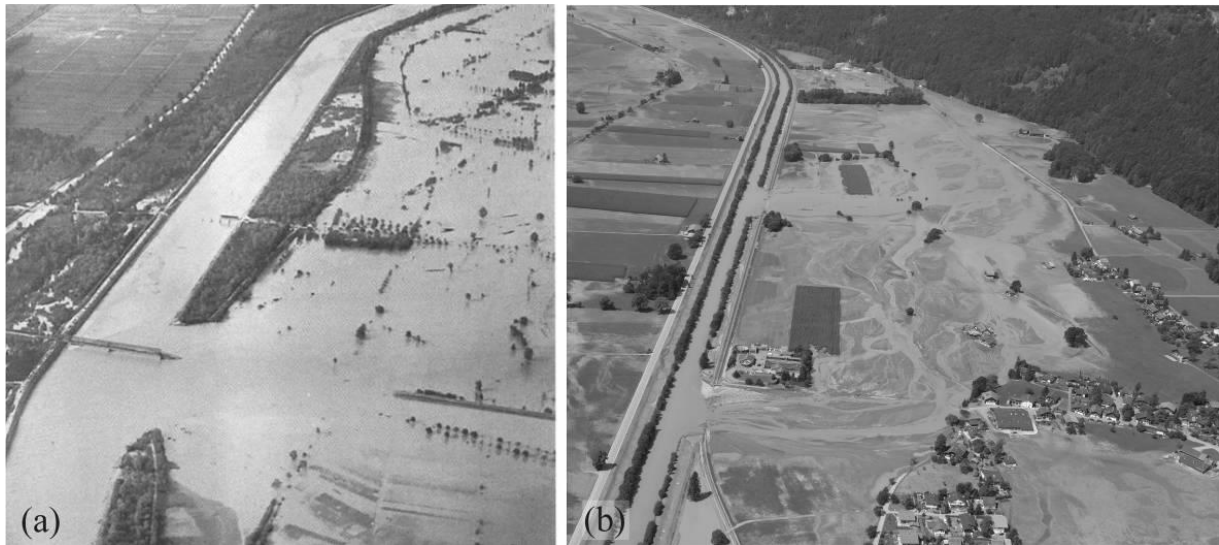
Figure 4 (a) Dike breach at Alpine Rhine River (Minor and Hager, 2004) and (b) Aare River (Photo: Swiss Air Force 2005)
