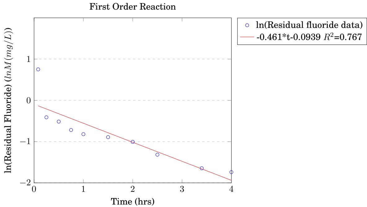
Figure B.2: First order reaction rate for fluoride adsorption by H_2SO_4 -treated AA
