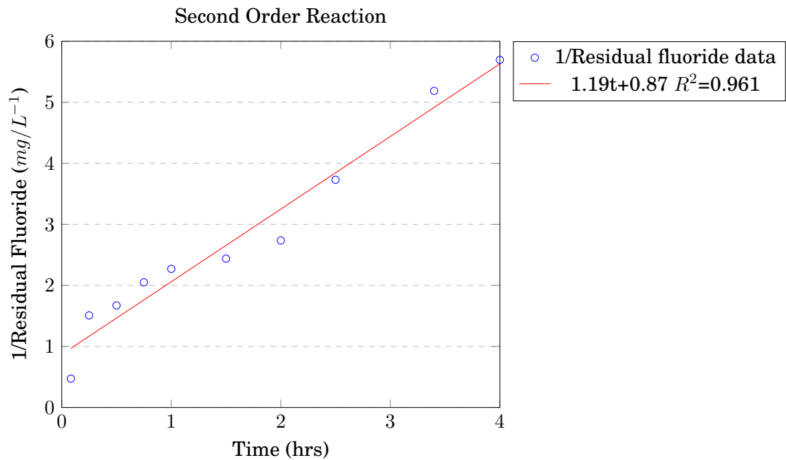
Figure B.3: Second order reaction rate for fluoride adsorption by H_2SO_4 -treated AA
