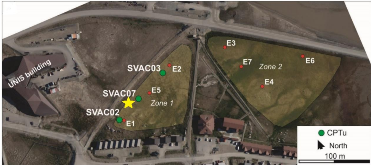
Figure 5-2 Detailed location of UNIS East site, red dots stands for boreholes, yellow star stands for the new Nunataryuk project site (Adapted from (Gilbertt, Instanes, Sinitsyn, & Aalberg, 2019))
