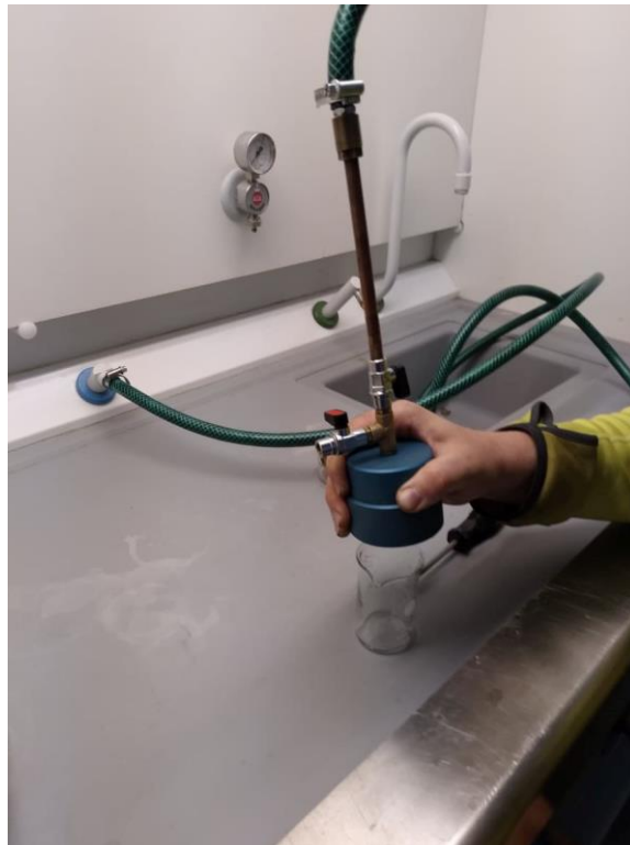
Figure 5-7 Device to extract liquid from the sample
