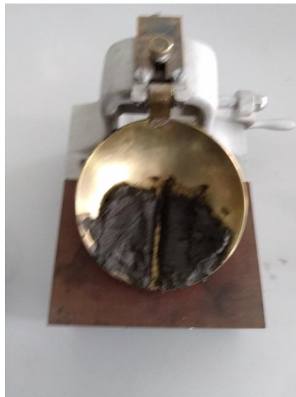
Figure 5-12 The Casagrande apparatus with soil sample and the groove
