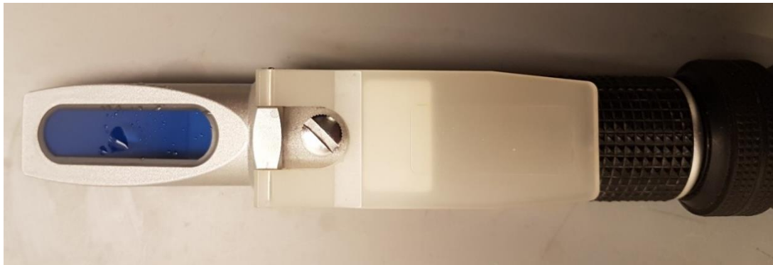
Figure 5-8 Refractometer with the liquid drop
