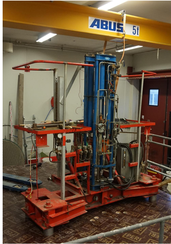
Figure A.37. The Borro bore rig on top of the scaffolding platform.
