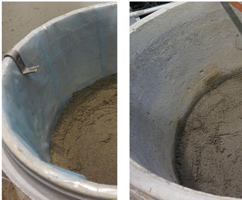
Figure A.22. Concrete wall roughness. Left: With plastic sheets, Right: Without.
