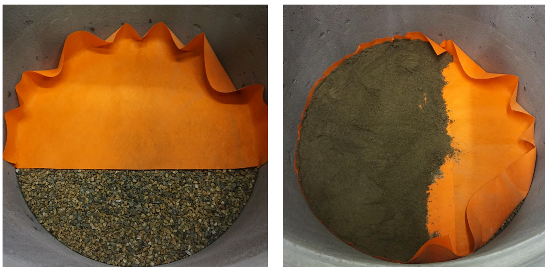
Figure A.21. Left: Gravel layer and filter, Right: Sand above the filter.
