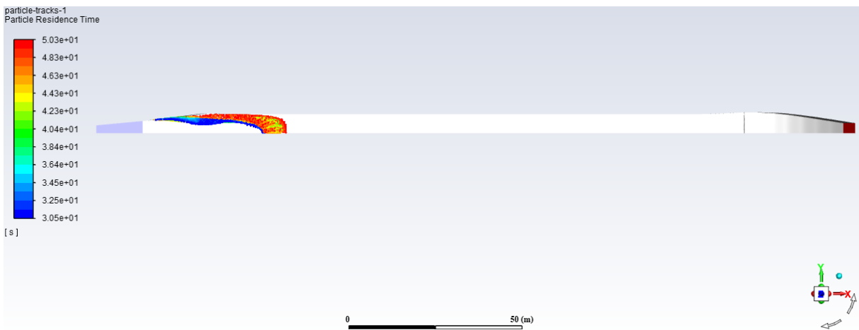
Figure 38: Injection of 1 mm particles - after 50 s.
