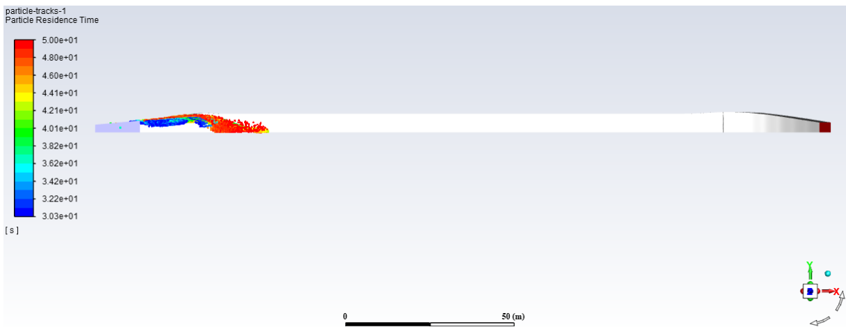
Figure 42: Injection of 0.3 mm particles - after 50 s.
