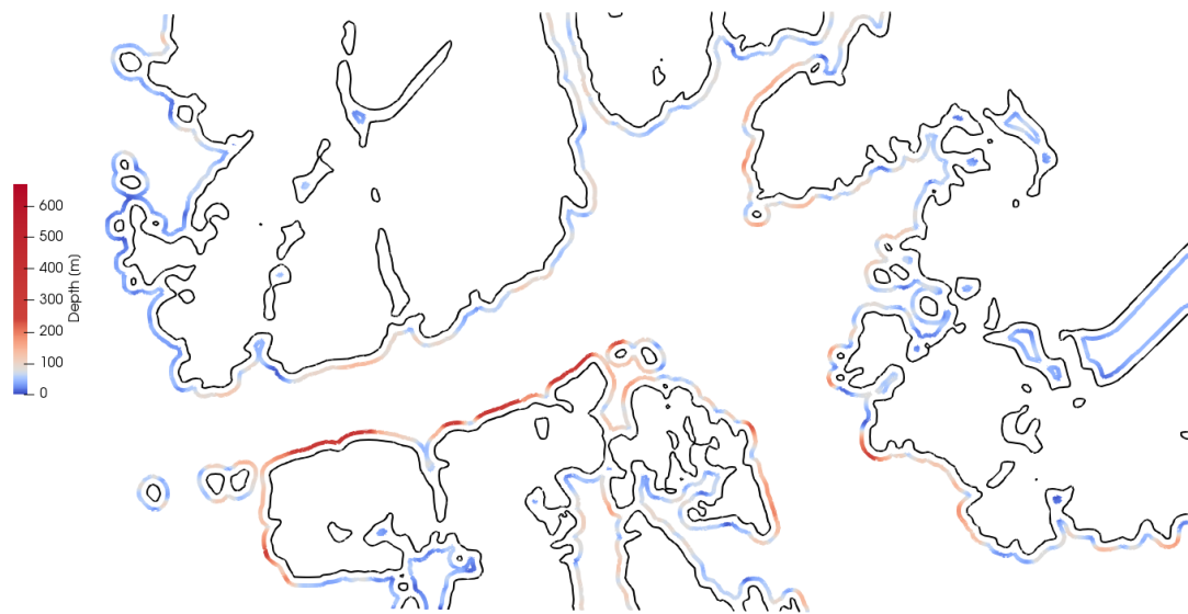
Figure 5.16: Depth at the start of the coastal relaxation zone. The coastline is represented by the black lines. Coastline damping distance = 200 m.
