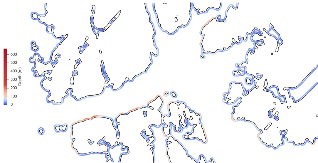
Figure 5.15: Depth at the start of the coastal relaxation zone. The coastline is represented by the black lines. Coastline damping distance = 120 m.
