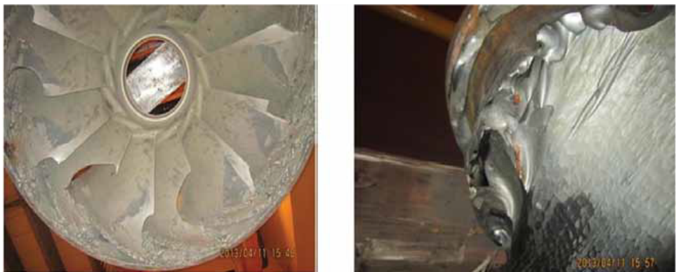
Figure 4.6: Erosion in runner and facing plates (Chhetry and Rana, 2015).
