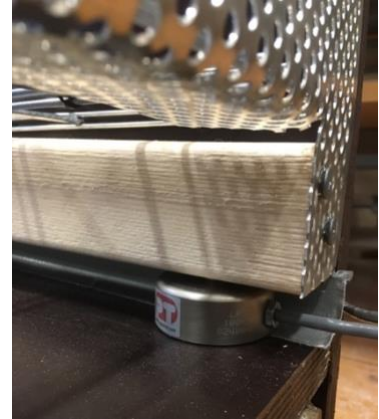
Figure 2. Load cell logging the weight loss of the trays due to moisture loss.
