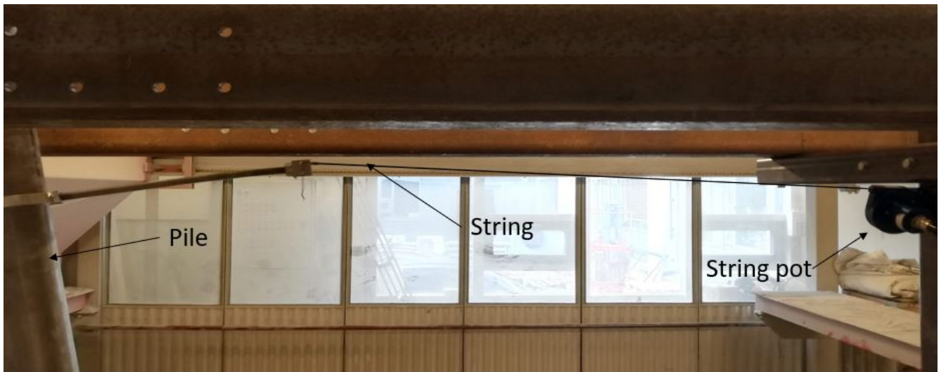
Figure 5.1: Picture illustrating the angle between string pot and pile.
