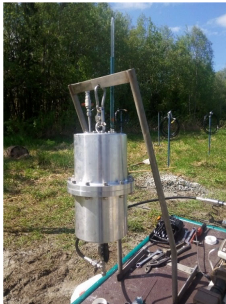
Figure 4- 9 Filled burette connected to upper outlet of the accumulator
