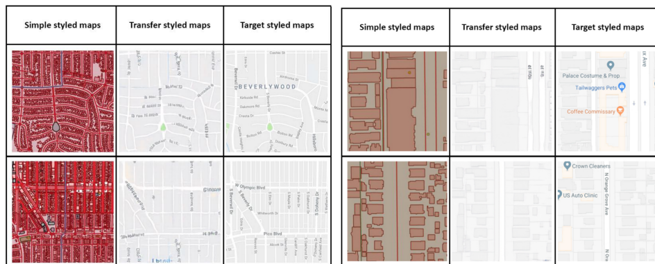
Figure 3.1: Map generalisation applied on simple styled maps using Pix2Pix, to the Google Maps equivalent, on zoom levels 15 (left) and 18 (right). Figure from the article.
