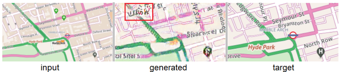
Figure 5.9: Mapnik-Michelin. Though buildings are deselected as intended, green roads are rendered with artifact-like elements, lacking in geometric precision too at intersections. The highlighted artifact is particularly bad and blocks other content. The H symbol is rendered badly too.
