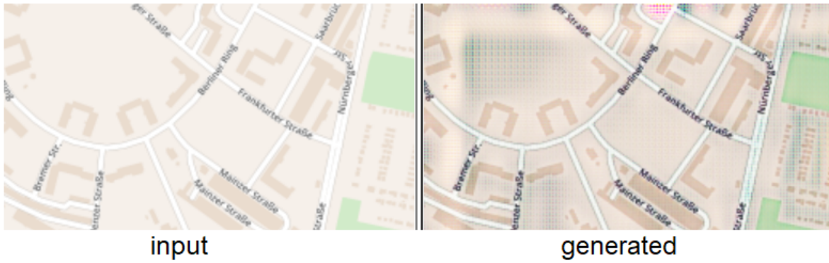
Figure 5.15: Severe failure on the Michelin dataset. A darker shade was applied. Grid artifacts showed up, despite the absence of transpose convolution in this architecture.
