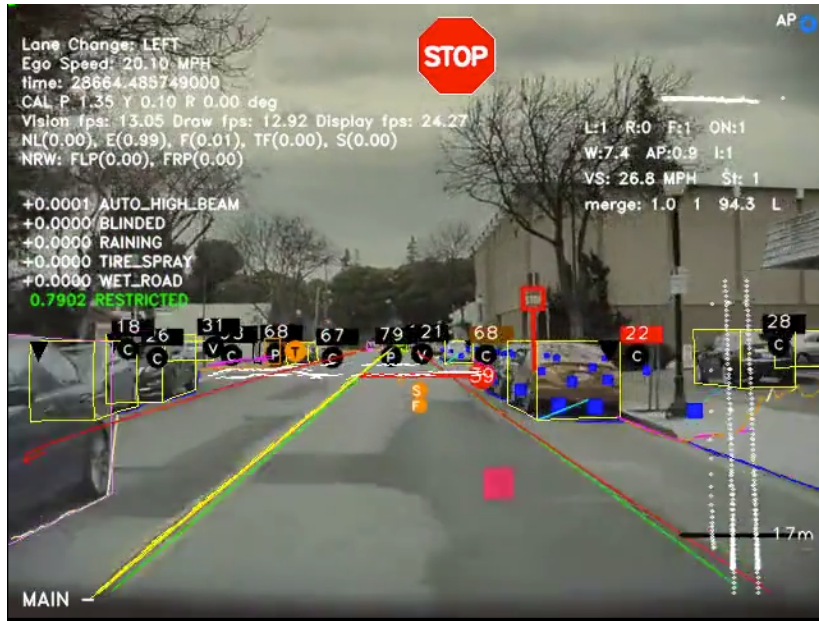
Figure 1.1: Demonstration of how Tesla Autopilot AI observes objects; screenshot from [Tes20]. Objects such as cars are marked with boxes, and the boundaries on the road are clearly marked with green, yellow and red lines. The stop sign is also detected, indicating a restricted area, as evidenced by the text on the left part of the image.
