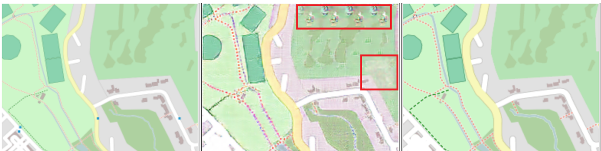
Figure 5.3: Left to right: input, generated, target image. Artifacts in OSM-no-labels can be seen in the middle image (zoom in). The generated images frequently have grid problems. The top box shows repeated artifacts, and the right box shows a blurred patch formed like an L rotated 180°, which is also an artifact.
