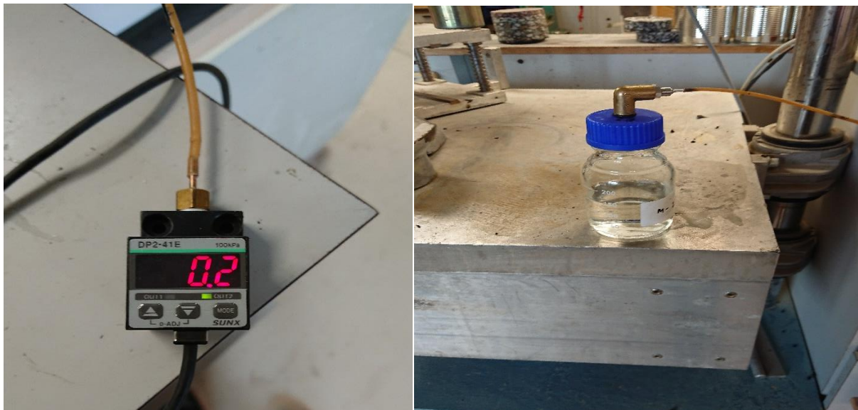
Figure 2: SUNX DP2-41E pressure sensor and bottle for measuring air and vapor pressure.
