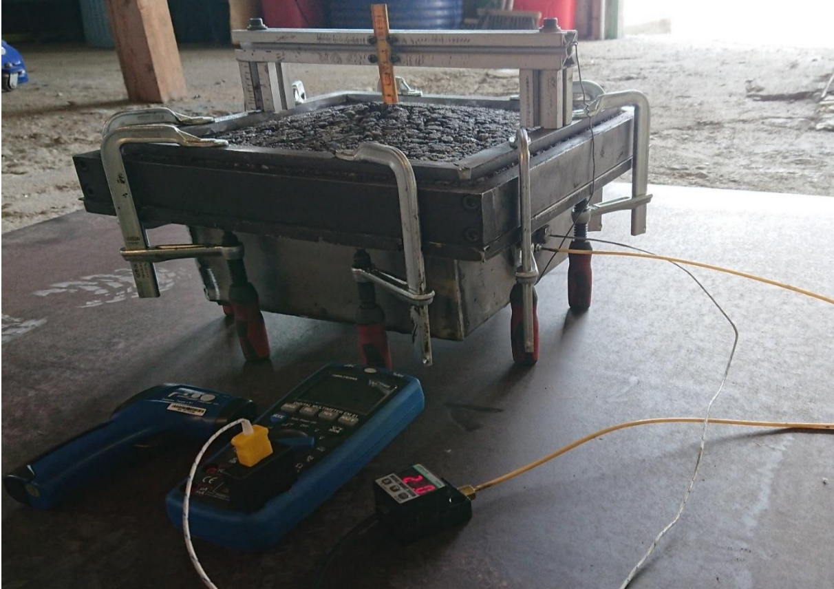
Figure 4: Complete blister test model with measuring equipment.
