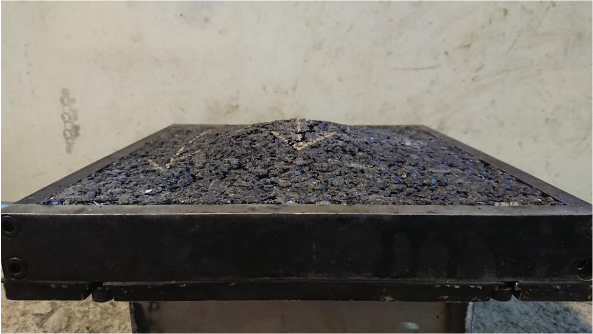
Figure 8: Blister from test 1 (4cm slab) with visible cracks on the top.
