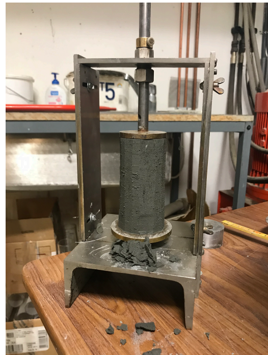
Figure 3.6: Sample after trimming on the sides
