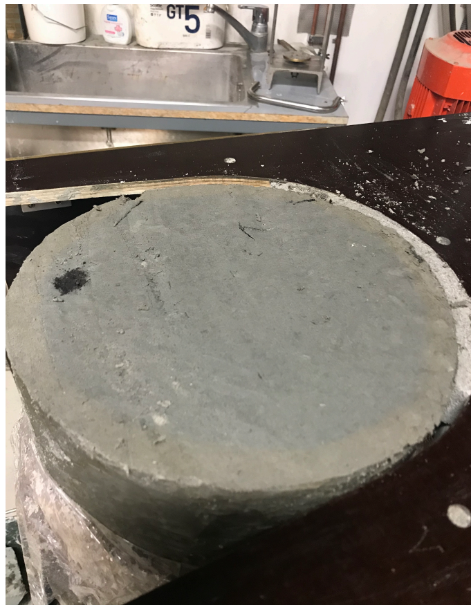
Figure 3.4: The block sample after trimming at the top
