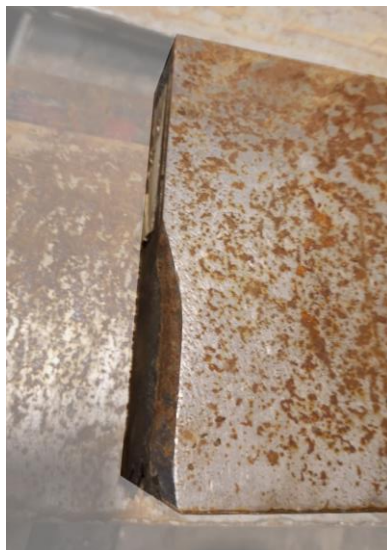
Figure 4.15: Steel chipping on Nordic Combi Double in one of the center plow positions
