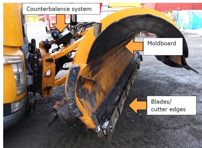
Figure 1.1: Main parts of a snowplow
