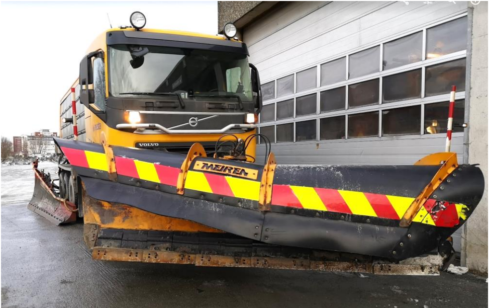
Figure 3.2: Plowing equipment used. Volvo truck, Meiren MSP plow and wing plow. Blade holders are the black parts behind/ directly above the blades.
