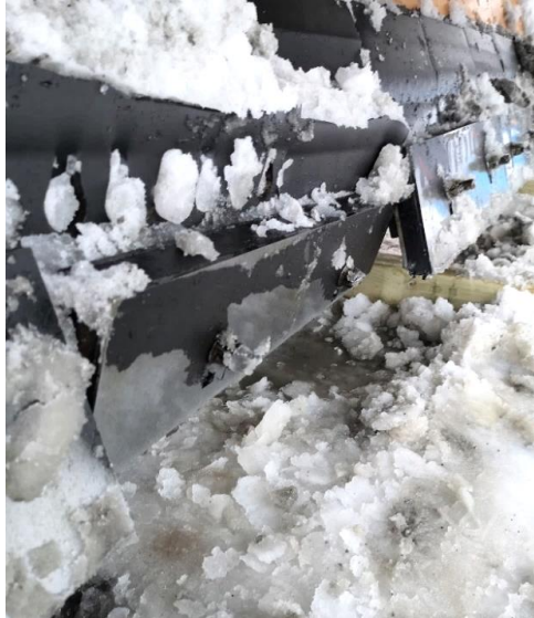
Figure 4.14: Broken blade holders
