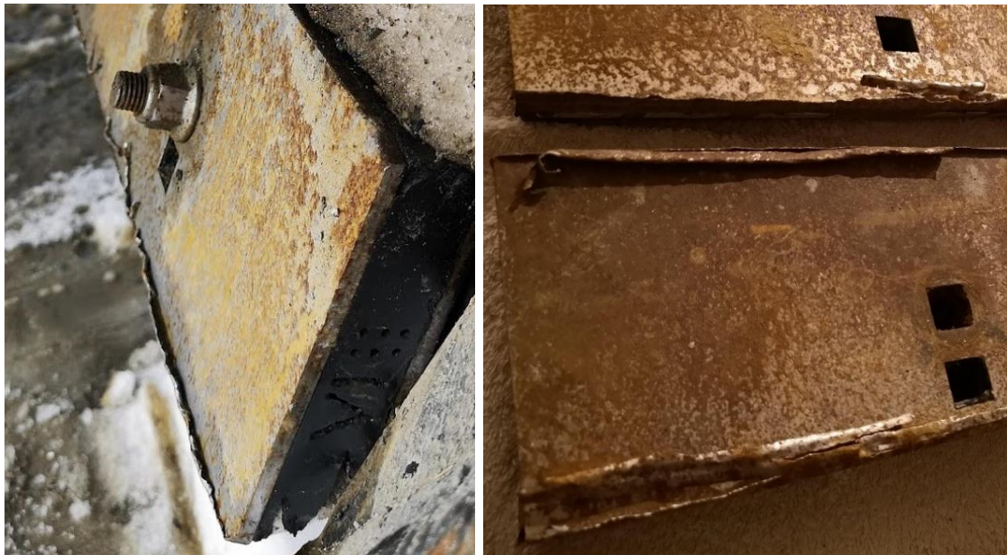
Figure 4.16: Steel buckling on blades
