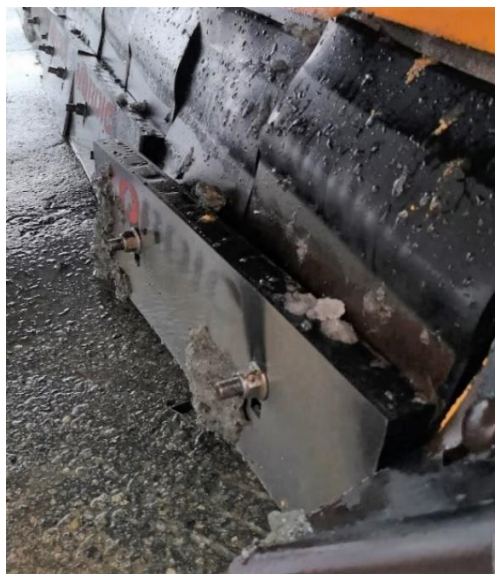
Figure 4.13: Bended blade, due to damaged blade holders
