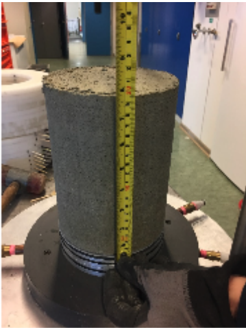
(c) Unmoulding and measurements on the frost cell
