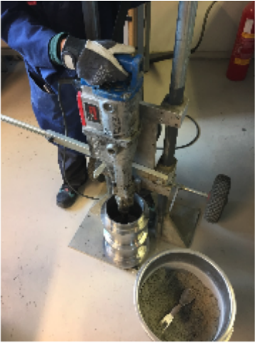
(a) Compaction of sample
