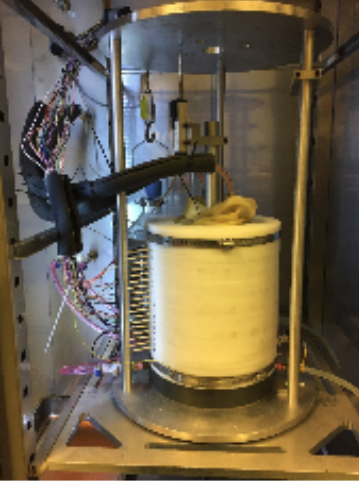
(f) Sample in frost cell, water and thermistors are plugged in.
