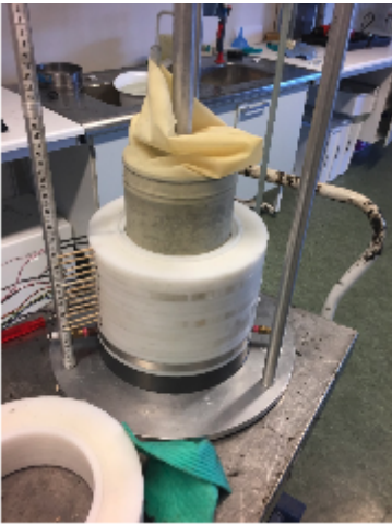
(e) Sample with the membrane and the rings.
