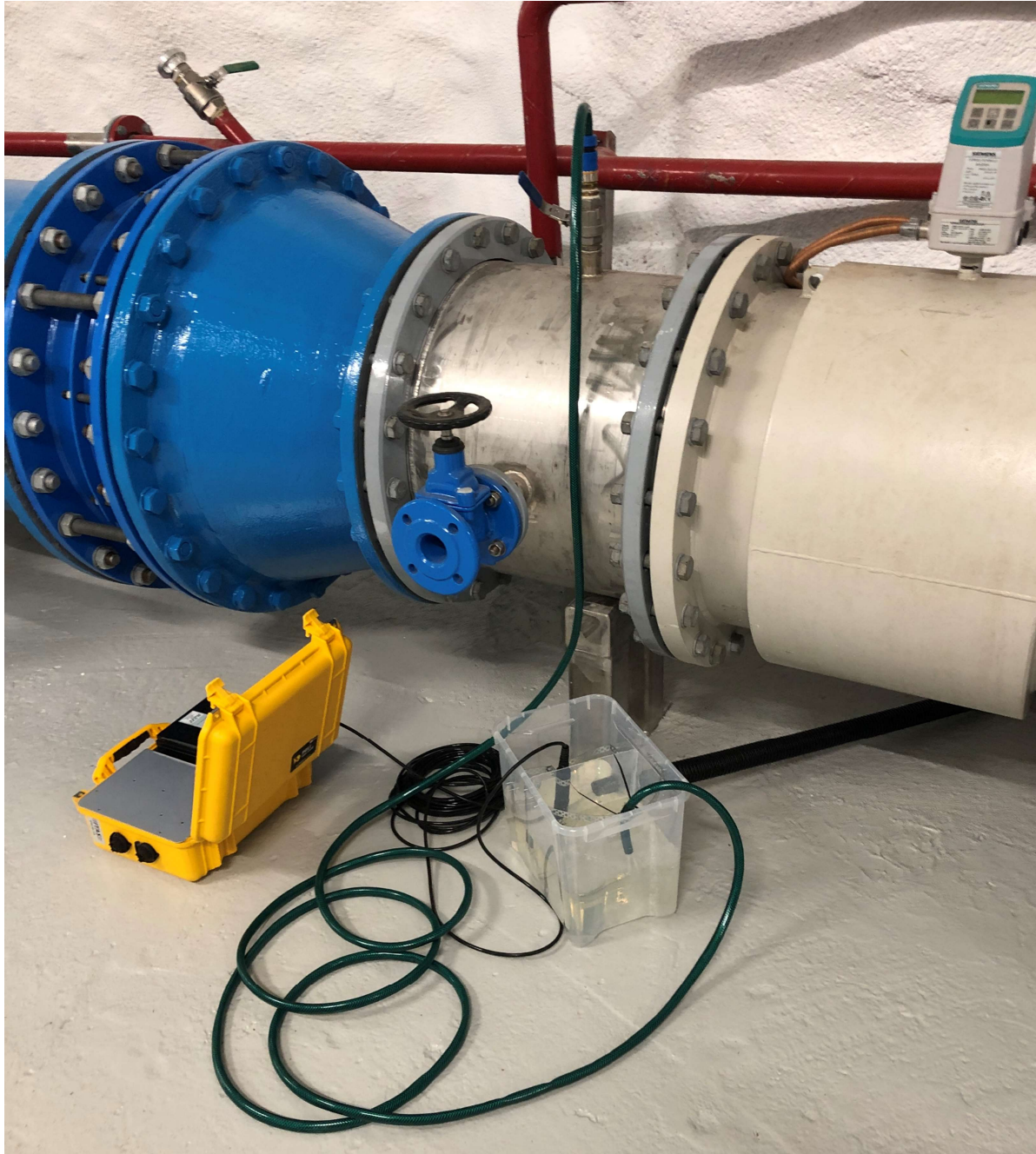
Figure 10: Photo of a data-logging kit installed and activated at one of the measurement stations
