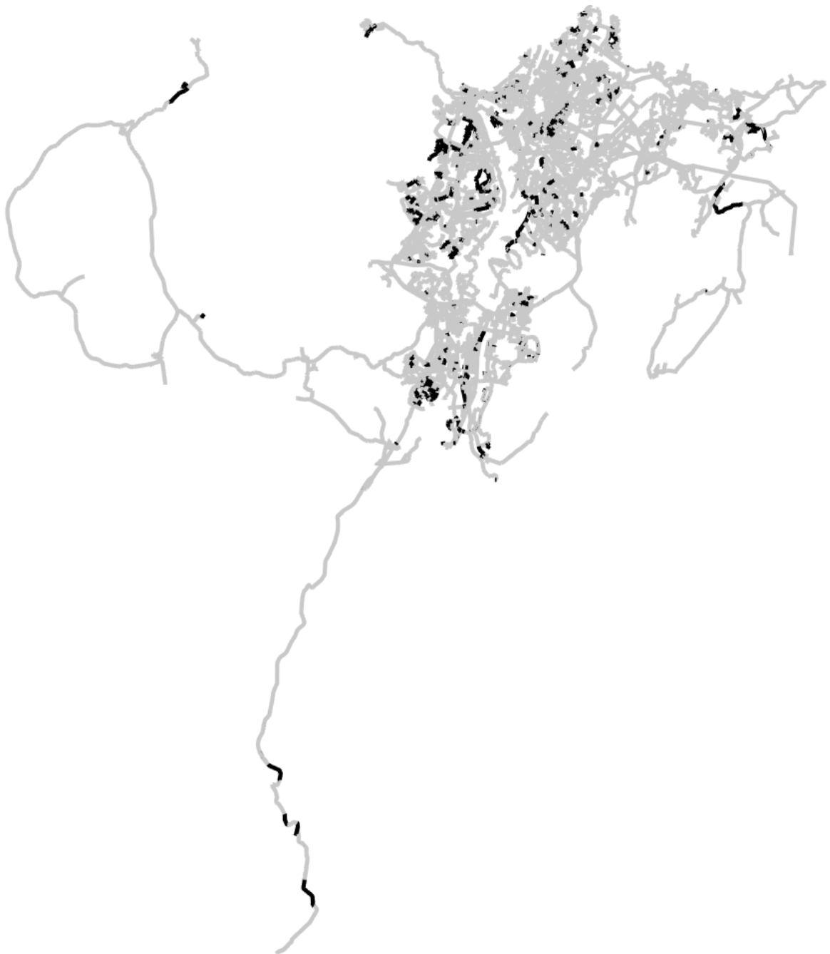
Figure 29: Overview map highlighting the pipes (in black) that had flow-reversals and met specified flow velocity requirements in the model
