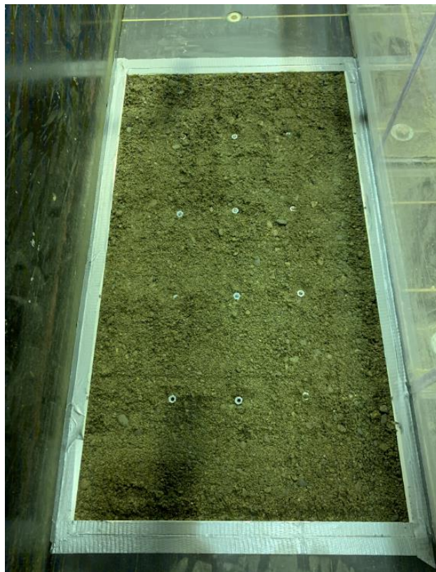
Figure 21 Picture of the erosion box in place in the channel.
