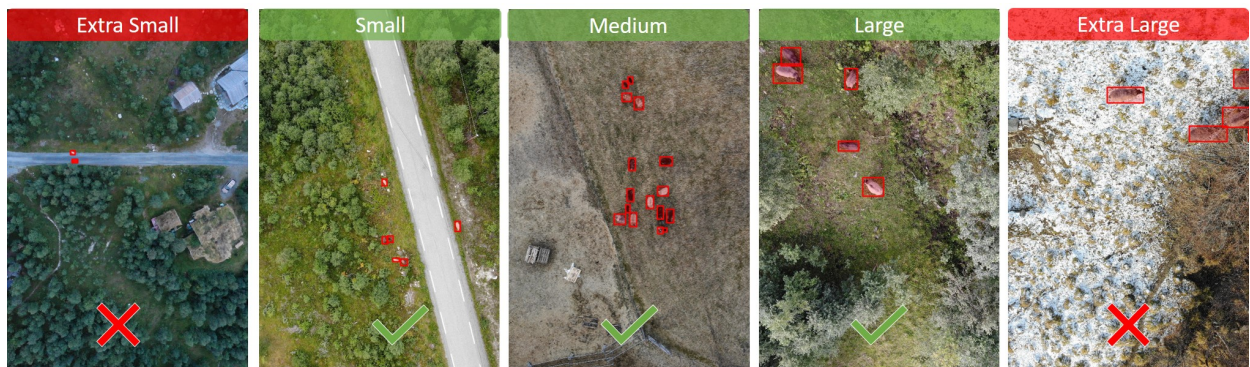
Figure 27: Images with too small or too large sheep are excluded from use. Accepted flight heights correspond to an approximate range of 14 to 85 meters.
