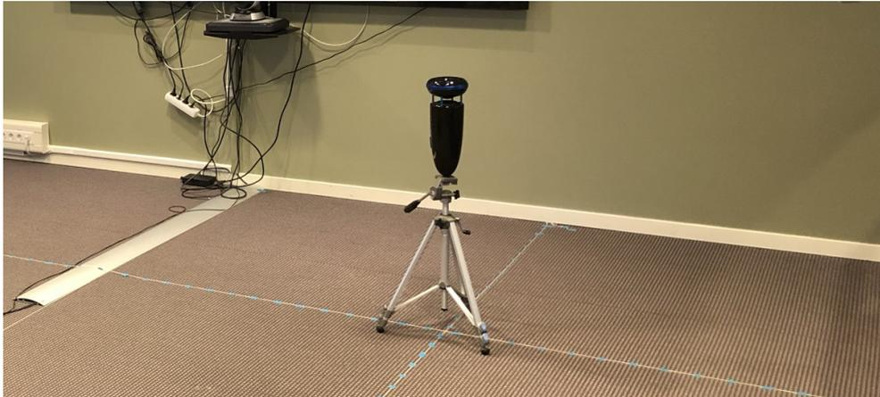
**Figure 3.8:** Source placed on an intersection between three nodal planes, as the acoustic center of the speaker is placed at a fourth of the room's height.
