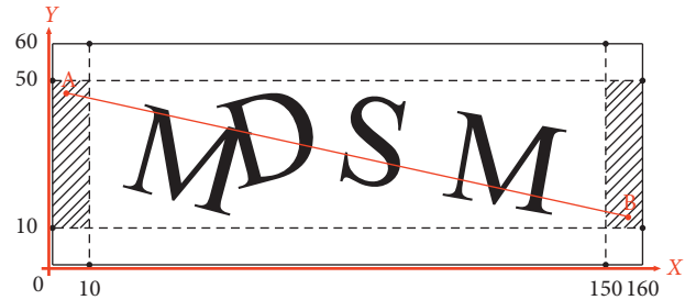
FIGURE 5: Principle of adding the occluding line. The CAPTCHA image size is 60 \times 160 . The abscissa represents the length, the ordinate represents the width, and the shading area represents the area where the left and right endpoints A and B of the occluding line are generated by the method.
